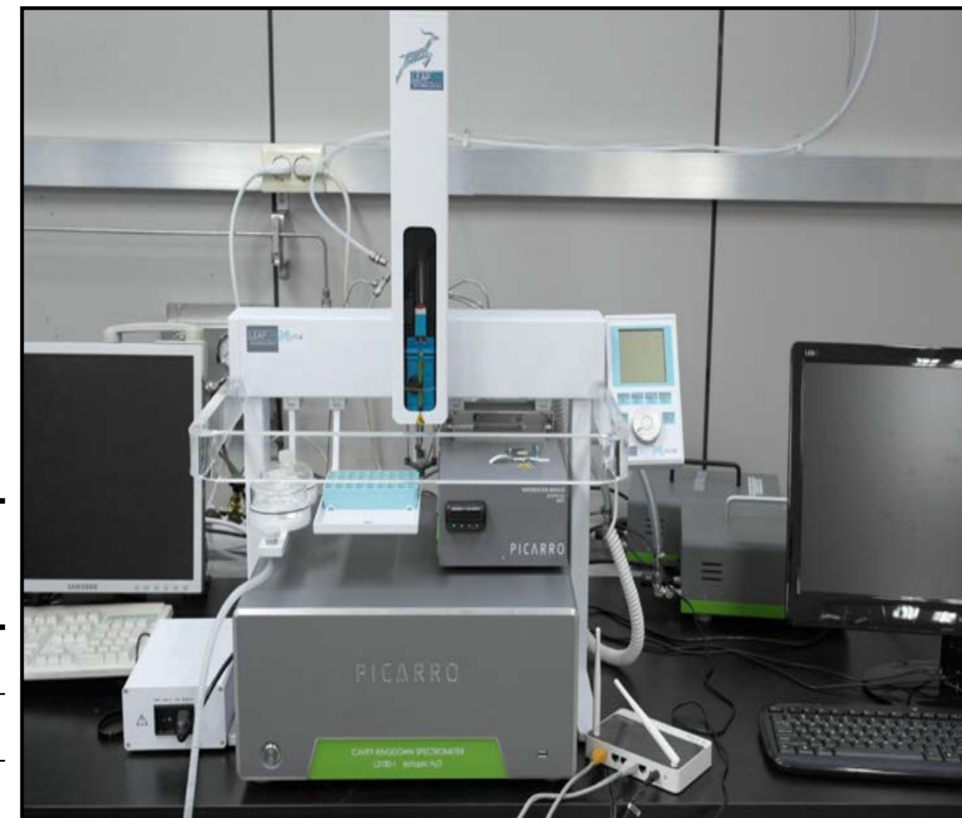
Fig. 3. WS-CRDS (Wavelength-Scanned Cavity Ring-Down Spectroscopy) used in study (L1102-I, Picarro, inc.). Precision : \delta^{18}O=0.15\text{‰} , \delta D=0.9\text{‰}
