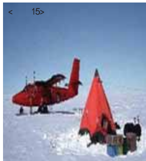
15 De Havilland Canada Twin Otters (DHC-6) 4 · (Wingspan) 19.8m · (Length) 15.7m · (Take off weight) 5,670kg · Twin Engine Turboprop · (Range) 1,435km · Cruising speed 130 knots 가
