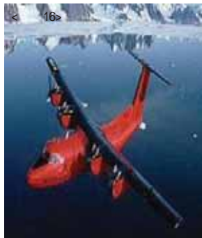
16 De Havilland Canada Dash-7 (DHC-7) 1 · (Wingspan) 28.4m · (Length) 24.5m · (Take off weight) 21,320kg · 4xTurboprop · (Range) 4,000km(1,500km fully loaded) · (Maximum speed) 230 knots · 50, 12~16 가
