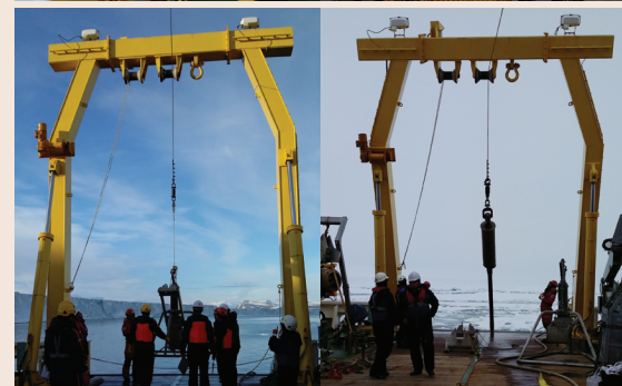
Box coring (left) and gravity coring (right) for collecting marine sediments. Ross Sea, Feb 2015.
