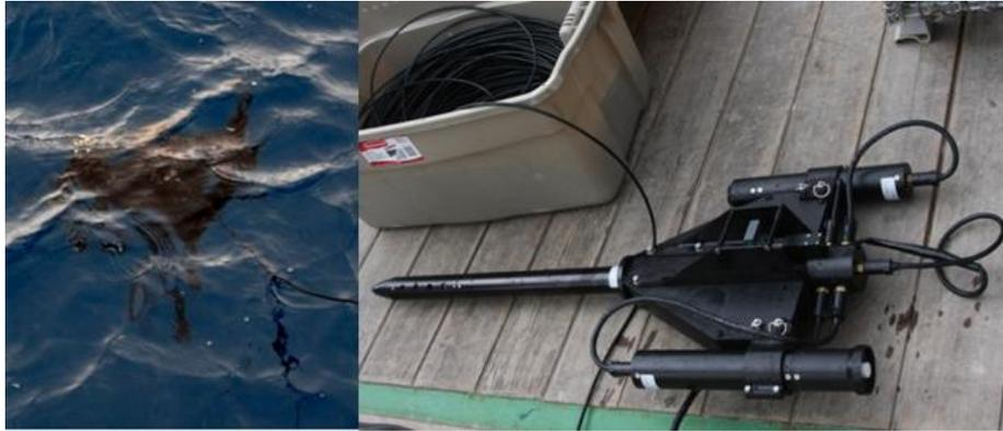
Figure 9.3: Hyper-spectroradiometer profiler (HPRO II, Satlantic Inc.,right figure) deployed in water(left figure).
