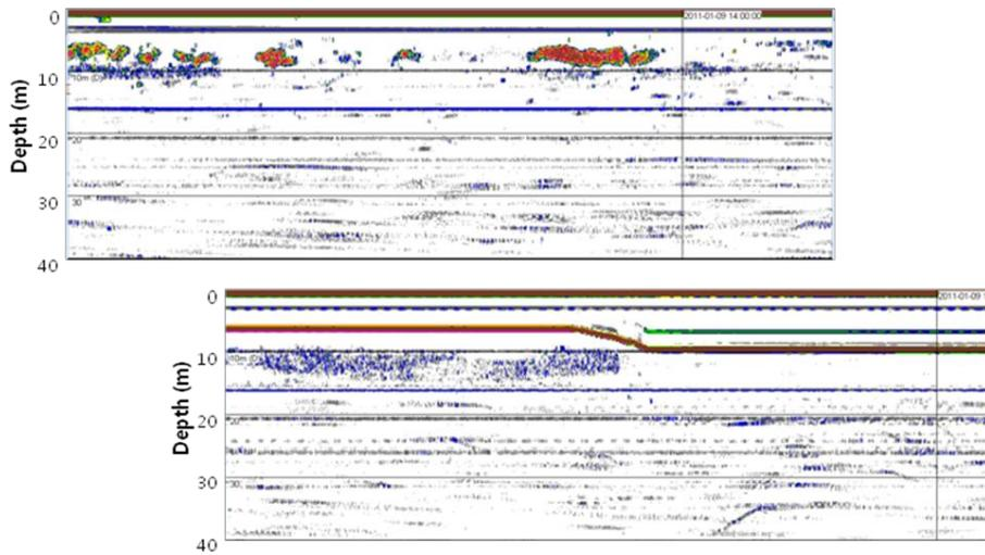
Figure 7.3: The example of hydroacoustic signal on the sea ice station (120 kHz).
