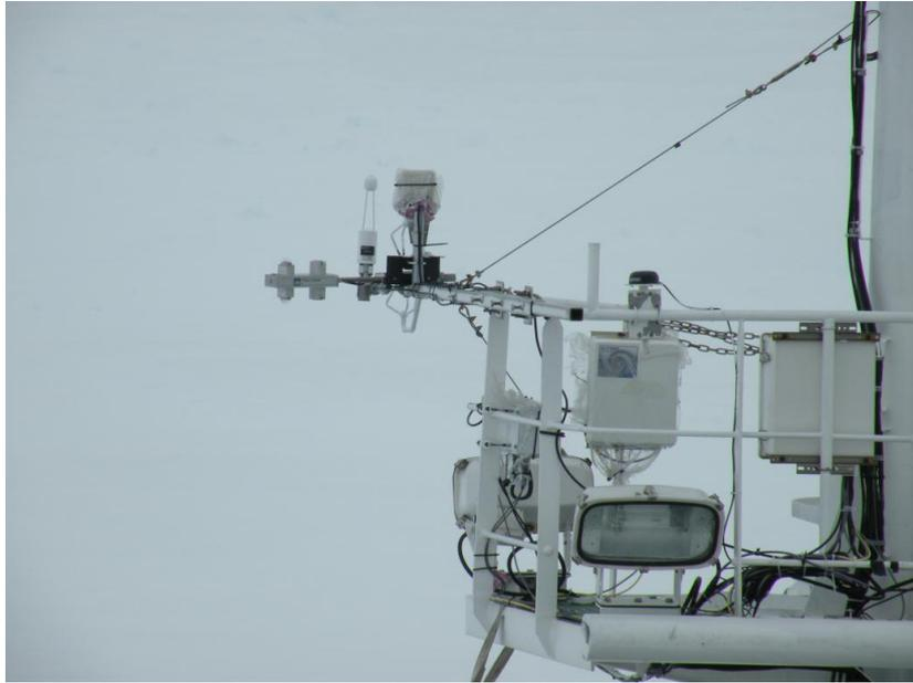
Figure 10.6: Eddy covariance system with motion sensor at the foremast of Araon
