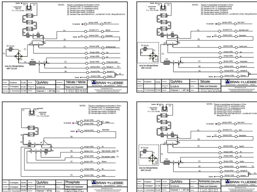
Figure 3.2: The manifold layout and flow chart of nutrient channels
