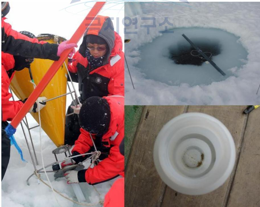
Figure 2.5: Deployment of small trap on the sea ice.
