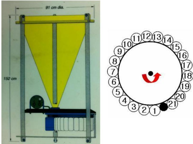
Figure 2.4: Sediment Trap schematic (model MARK 78G) and bottle rotation.
