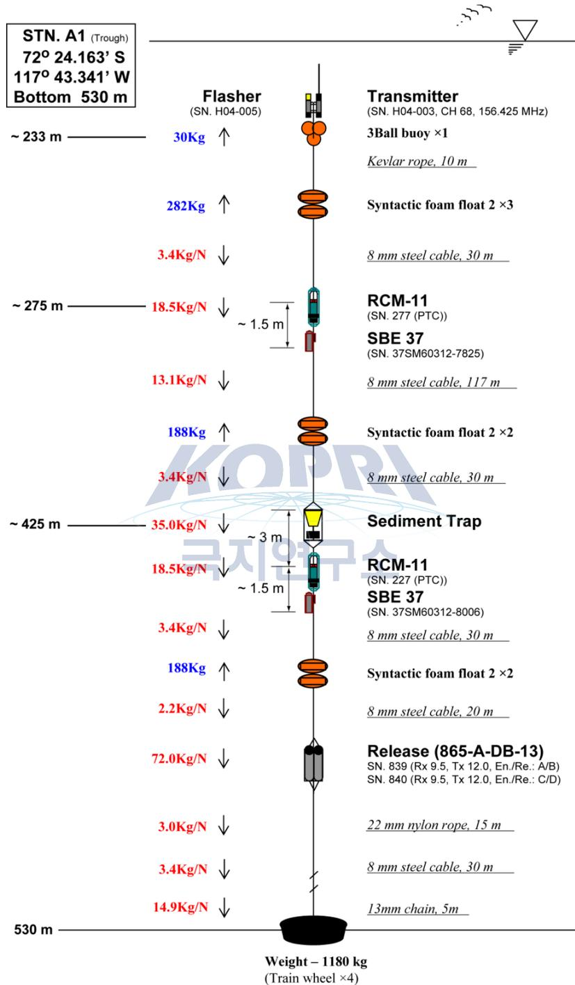
Figure 2.2: Mooring configuration at station of A1 (trough site).
