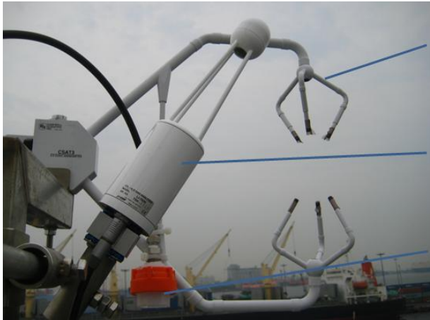
Figure 1.2 Open-path eddy covariance at the foremast of Araon.
