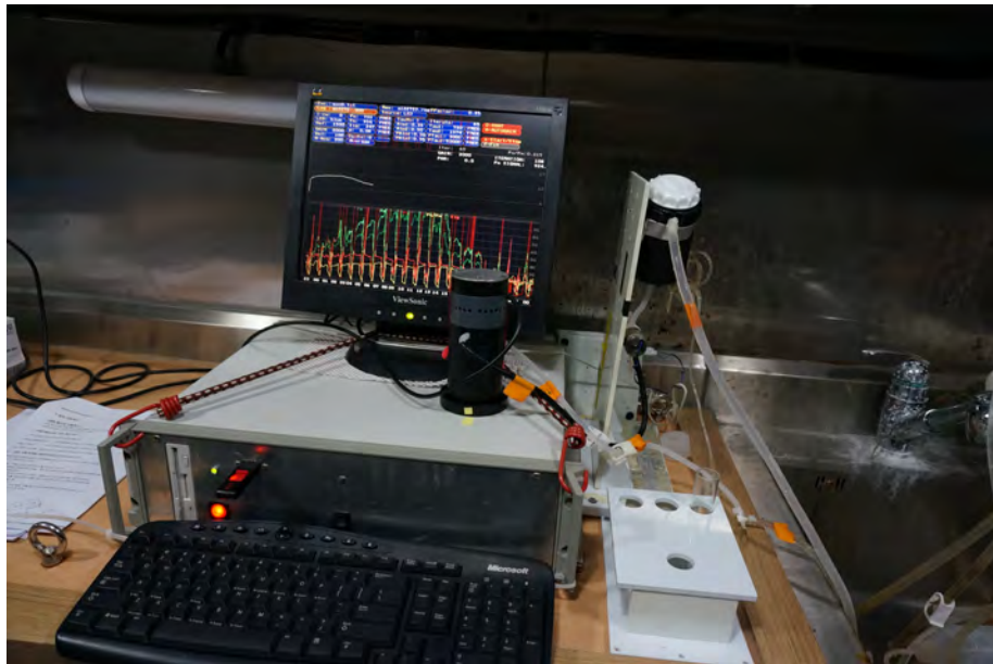
Figure 3.5: A Fluorescence Induction and Relaxation (FIRe 2) system which was installed on the ARAON.
