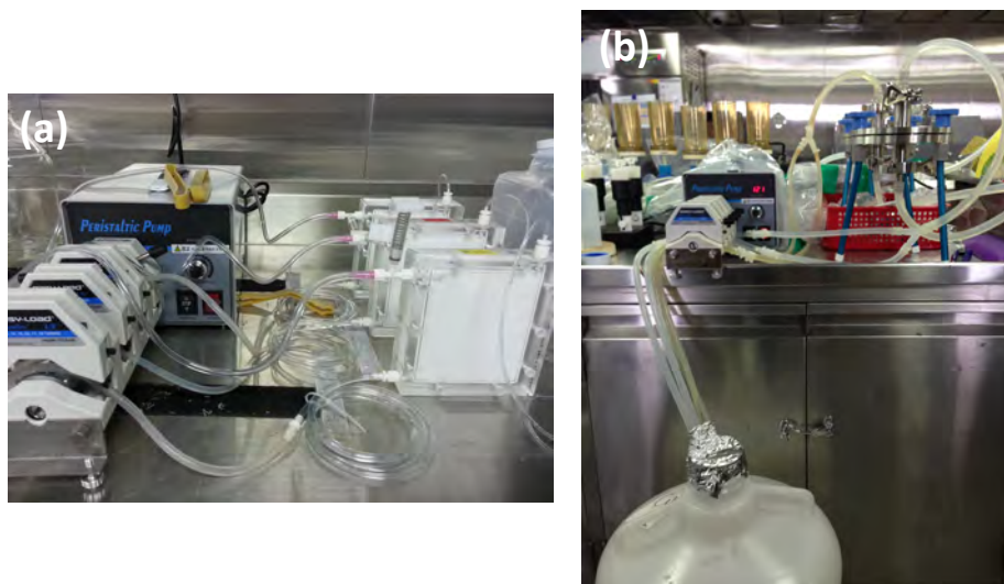
Figure 3.11: Photos of (a) a tangential flow filtration system and (b) a large volume seawater filtration system used in the present study.
