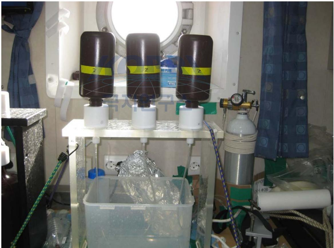
Figure 2.13 Nitrogen gas purging system for collecting DOC and POC.
