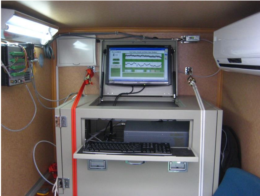
Fig. 1.4. Cavity ring-down spectroscopy (CRDS) analyzer in the O2Deck shelter (Adapted from 2013 ARA04C cruise report).
