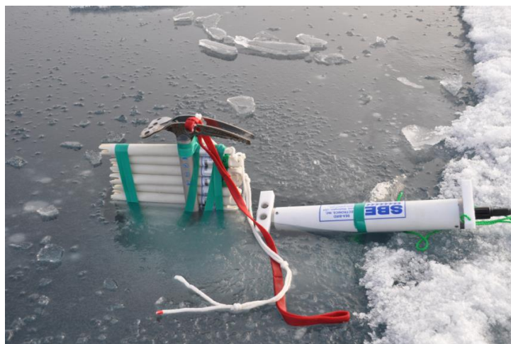
Fig. 2.6. TUMSAT CTD profiling measurements on the sea ice floe (upper) and TUMSAT melt pond survey using SBE56 and SBE37 (lower).
