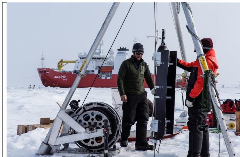
Fig. 11.11. Preparing to lower ITP-V 80 into the 24" diameter hole.
