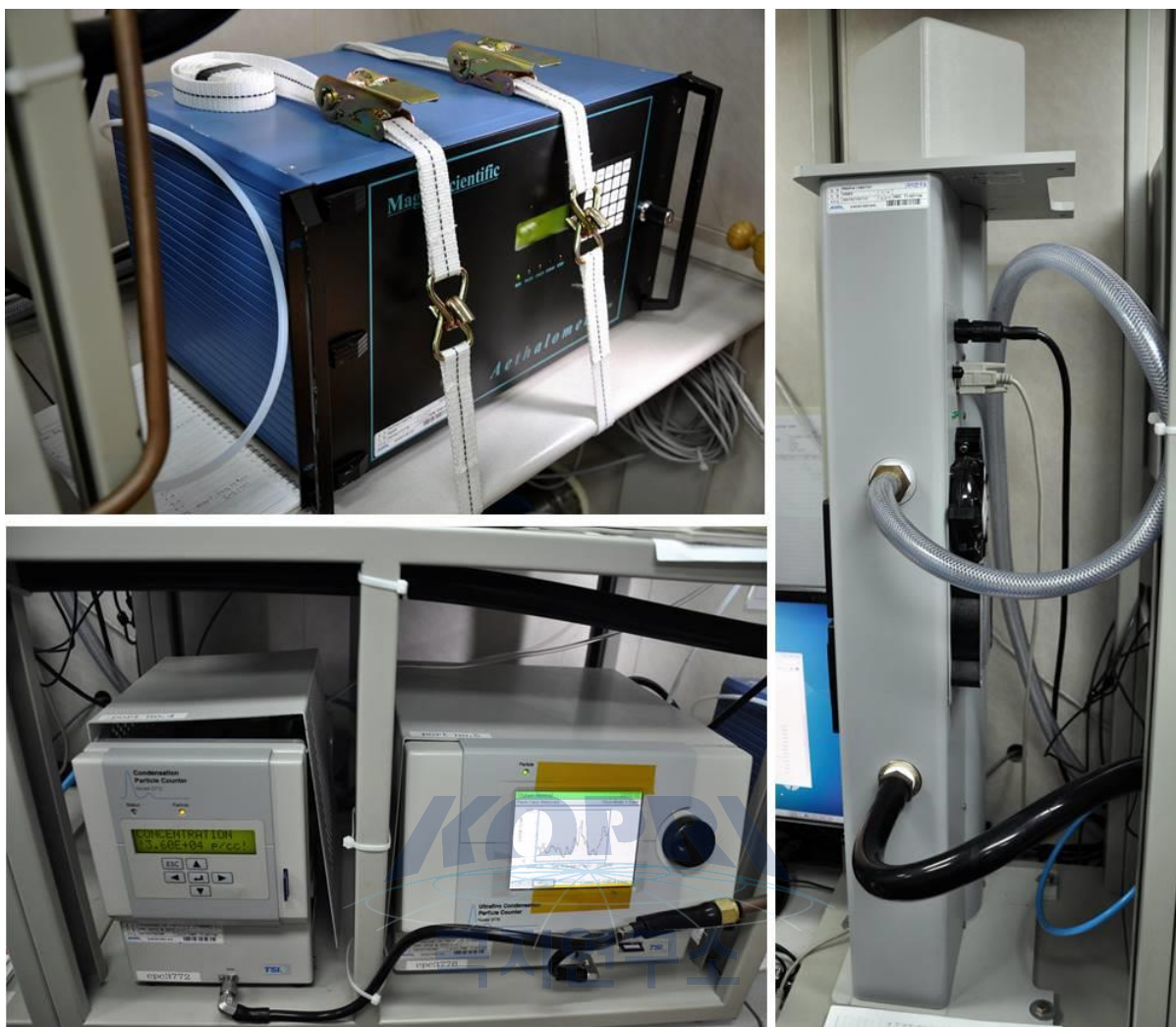
Fig. 1.8. Aerosol measuring instruments: (Up-left) Aethalometer, (Bottom-left) Condensation Particle Counters (CPC3772 and CPC3776), and (Right) Nephelometer.
