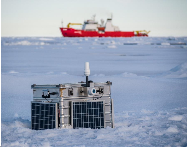
Fig. 11.8. A Seismic Wave Buoy (234) installed 1.2 km NW of Araon.
