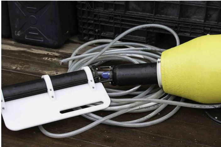
Fig. 7.4. SWIFT15 post recovery. The top and bottom halves have been separated by some severe impact, and are held together by only a thin interconnect cable. From the telemetered data and from the initial surface angle, it is certain that this damage was inflicted during the drift.
