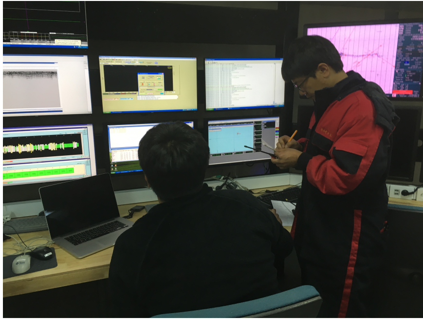
Figure 2.5. The seismic survey control system in the Main Dry Lab. Navigation, airgun controller, bird controller, recording system and quality control system are shown.
