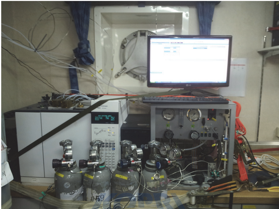
Figure 6.3. Gas chromatograph system for the measurement of the greenhouse gases including \text{CH}_4 , \text{CO}_2 , and \text{N}_2\text{O} .
