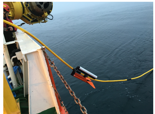
Figure 2.4. (left) Airgun array is launched into the sea. A float (red color tube) maintains the source depth as 6 meter in the water, (right) Launching the streamer with the cable leveler (bird).
