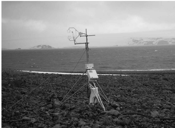
Fig. 1. (a) Landscape of King Sejong Station (top) and (b) Eddy covariance system (bottom).
