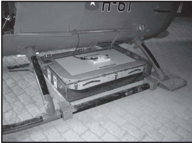
**Fig. 2.** The shielded 100-MHz ground-penetrating radar unit mounted between the skids of a helicopter in the broadside transverse electric antenna arrangement. Using this unit, a 10-ns radar pulse was generated at 35-ms intervals and received for 3700 ns at each shot point along Profiles A1–A3 across portions of the Fourcade Glacier.
