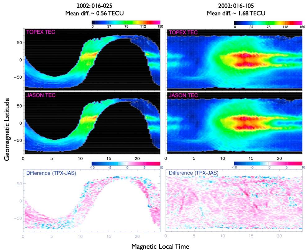
**Figure 4.** The TOPEX and JASON-1 TEC maps and their differences map in the geomagnetic latitude and local time coordinate for (first column) a 10 day cycle and (second column) a 90 day period in 2002. It takes about 90 days to cover a full 24 h of local time. Each column presents the TEC maps from (top row) TOPEX, (middle row) JASON, and their difference (TOPEX TEC – JASON TEC, bottom). The color scale ranges from 0 to 150 TECU for TEC maps and –10 to 10 TECU for difference map.
