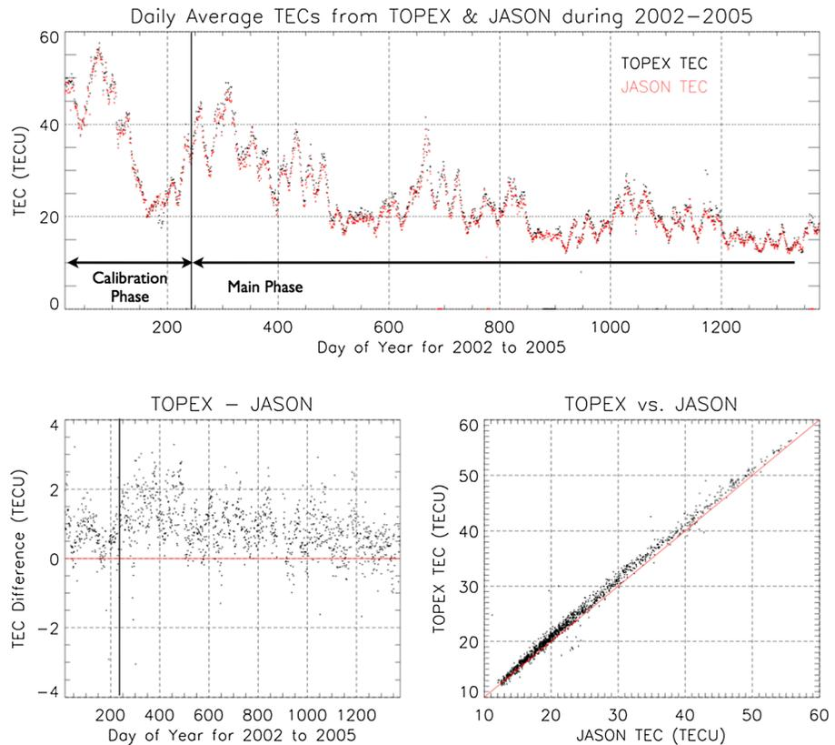
**Figure 3.** The daily mean TECs versus the day of year for the overlap period of the two satellite missions from 2002 to 2005. (bottom left) The differences between the two TECs are also displayed. (bottom right) TOPEX TEC versus JASON TEC in TECU are shown.
