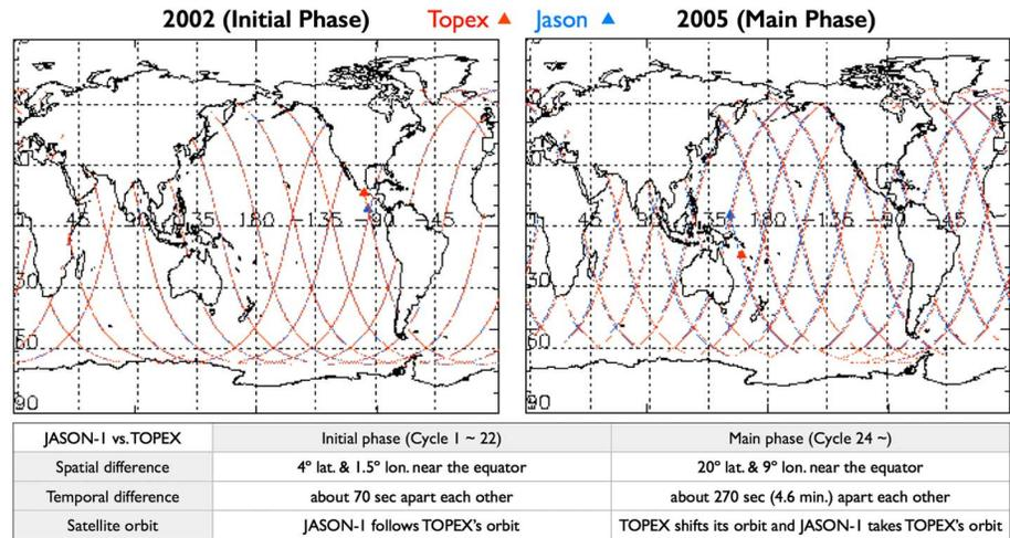
**Figure 2.** Spatial discrepancies between the TOPEX (red filled  $\Delta$ ) and JASON-1 (blue filled  $\Delta$ ) satellite orbits for (left) initial calibration phase and (right) main phase of the JASON-1 satellite mission. The red (TOPEX) and blue (JASON-1) dotted lines are the ground tracks of the satellite orbits. The table below the maps shows the differences between the two satellite orbits for the initial and main phases.
