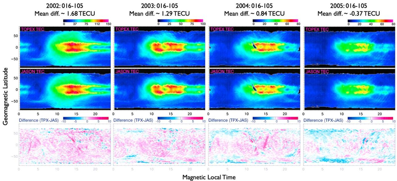
**Figure 5.** The global ionospheric TEC maps for each 90 day period between (left to right) 2002 and 2005 in the same format in Figure 4 (second column). Note that the color scales for the TEC maps are different for each year; 0~150 TECU for 2002, 0~100 TECU for 2003, and 0~80 TECU for 2004 and 2005. But the color scales for difference maps are all the same, -10~10 TECU.
