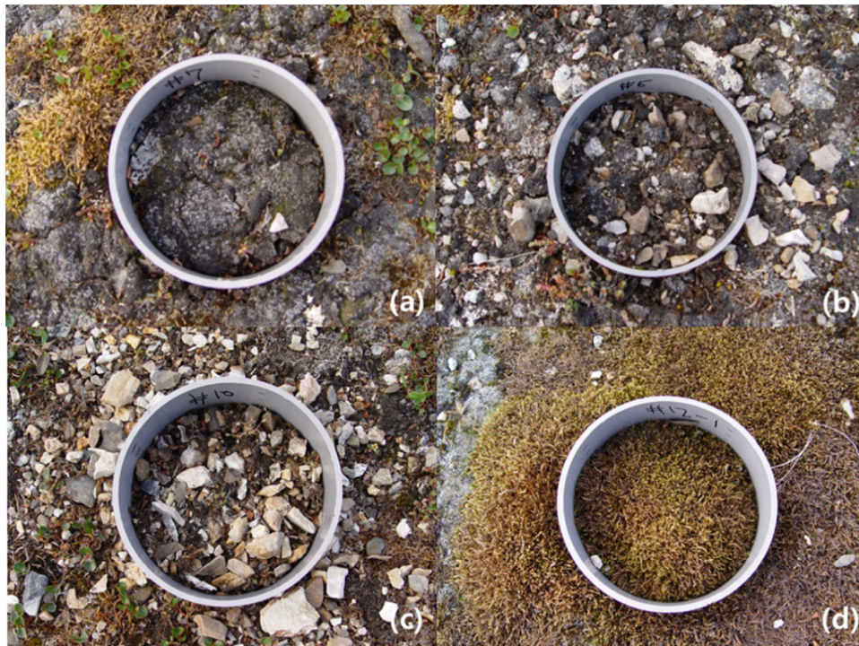
Fig. 2. Photo shots of soil CO 2 efflux measurements of biological soil crust with black color, Nos. 7 (a), 6 (b), and 10 (c), and a photo shot of moss CO 2 efflux, No. 19 (d) in PVC collar (10.6 cm in diameter and 8 cm in height).
