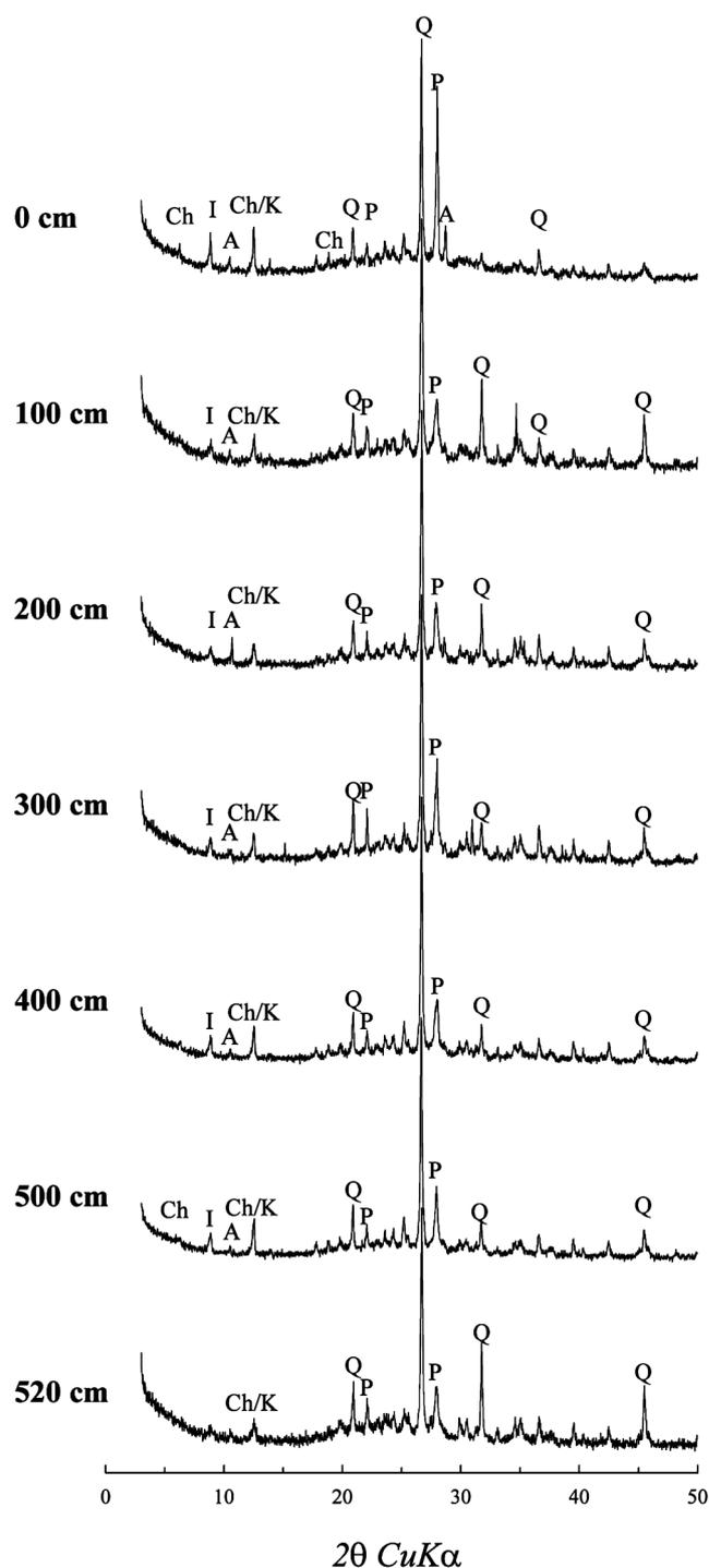
**Figure 5.** X-ray diffraction diagram of powdered bulk sediment samples of core GC02-SOI03. A, amphibole; Ch, chlorite; Ch/K, chlorite and/or kaolinite; I, illite; P, plagioclase; Q, quartz
