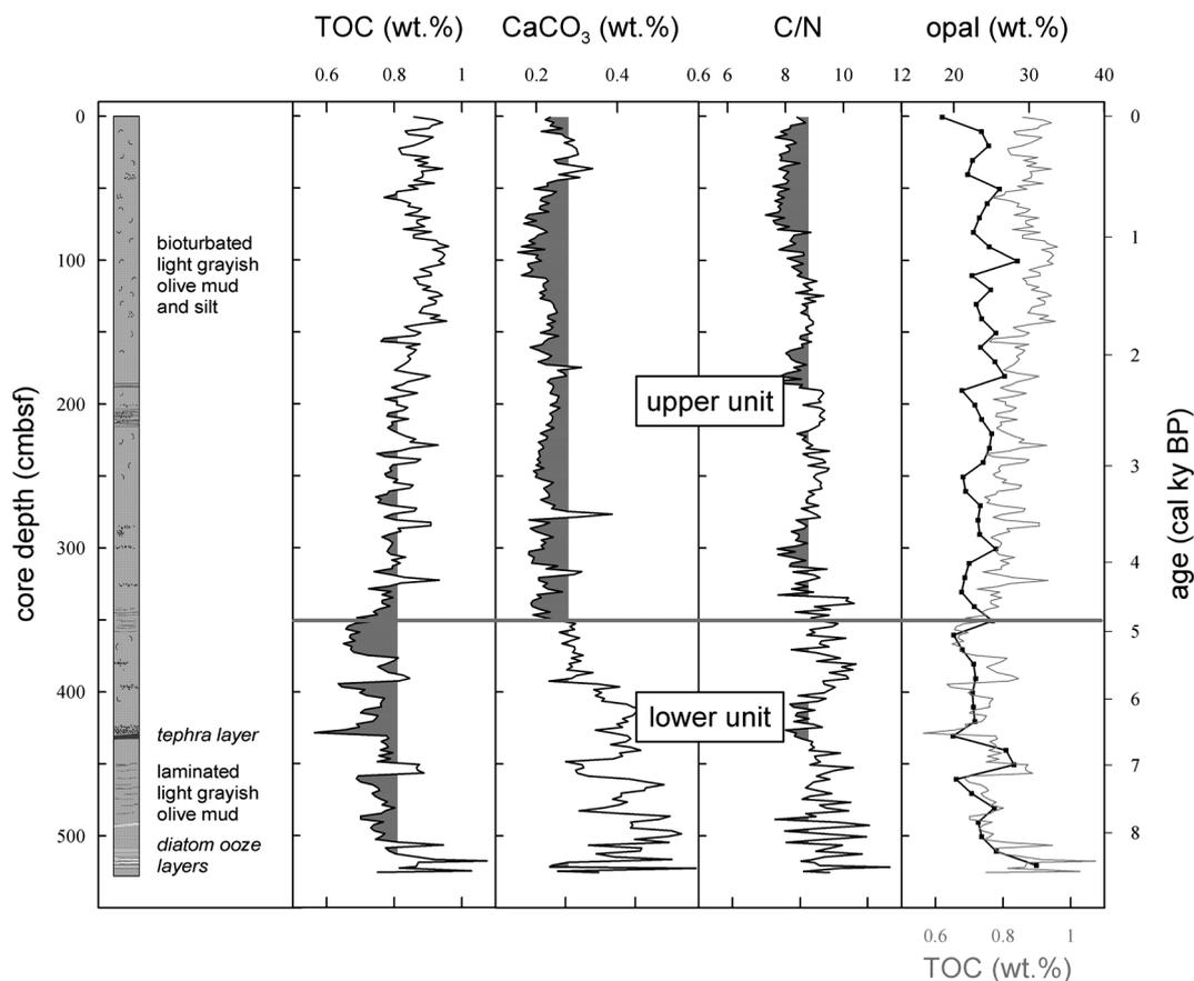
**Figure 6.** Total organic carbon content (TOC),  $\text{CaCO}_3$  content, TOC/total nitrogen ratio (C/N), and biogenic silica content (opal) of core GC02-SOI03
