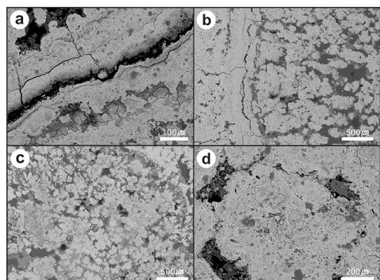
**Fig. 4.** BEI images of microstructure in Mn nodules from the East Siberian Sea. (a) columnar, (b) boundary between columnar and cuspat-globular (c) cuspat-globular, (d) massive.
