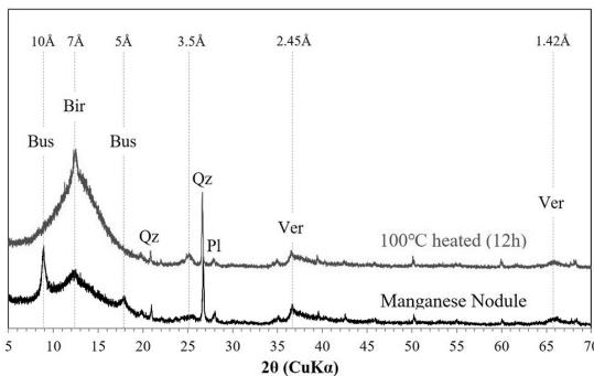
**Fig. 2.** XRD patterns of untreated and heated (100°C, 12 h) Mn nodule. Bir; birnessite, Bus; buserite, Pl; plagioclase, Qz; quartz, Ver; vernadite.
