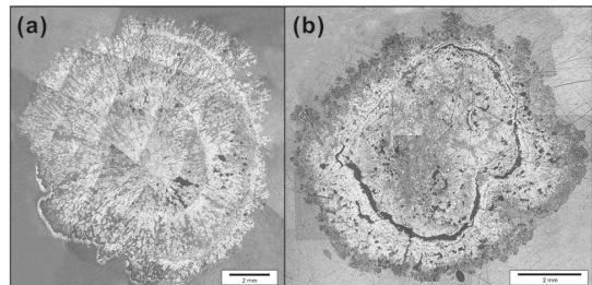
**Fig. 3.** Microphotographs of textures in Mn nodules. (a) radiated texture, (b) massive (inner) and layered (outer) textures.
