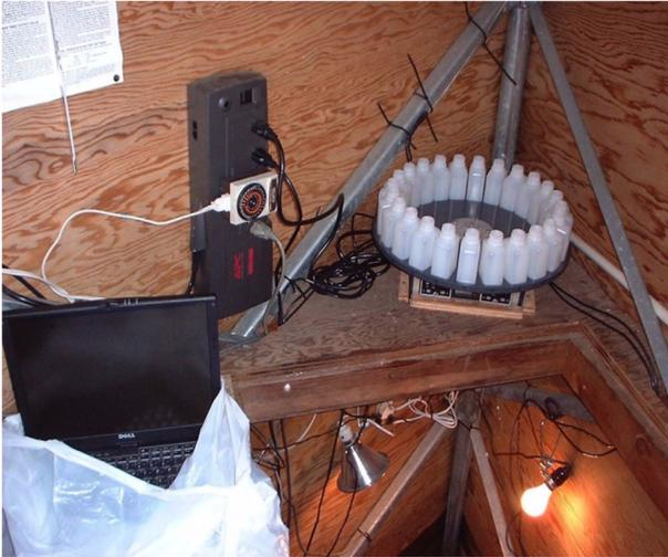
Fig. 1. Device for sampling snowmelt.
