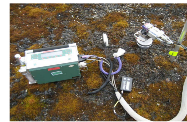
Figure 5. Chamber measurement system of soil CO 2 emission
