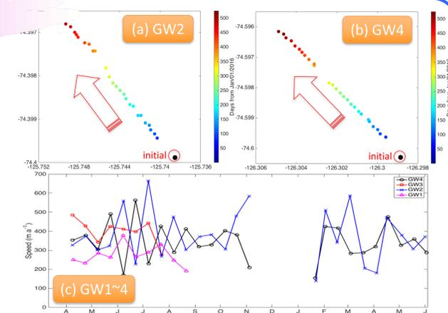
Fig.7 GPS monitoring: ice movement over 7 days at GW2 (a) and GW4 (b), and ice speed averaged over 15 days (c).
