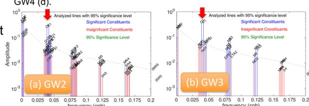
Fig.10 Tidal harmonic analysis of melt rates at GW2 (a) and GW3 (b).
