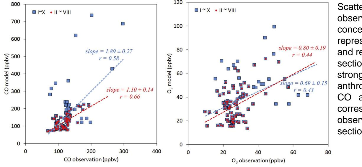
Scatter plots between the observed and modeled CO and  $O_3$ concentrations. Blue squares represent all of the 6-h mean data and red dots exclude the data from section I, IX and X that were strongly influenced by anthropogenic emissions. For both CO and  $O_3$ , the model results better correspond the to observations when the data from section I, IX and X are excluded.
