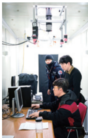
Figure 1. Optical observatory of space environment at which an all sky camera and Fabry-Perot interferometer are installed for measurements of airglow emissions to monitor atmospheric waves and thermospheric winds and temperature, respectively.
