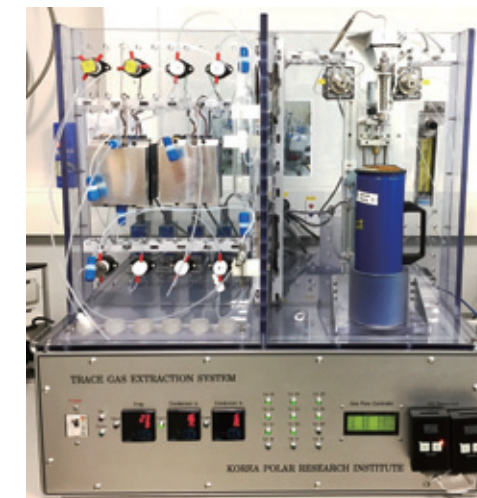
Figure 1. Trace gas extraction system for the analysis of dissolved \text{N}_2\text{O} .
