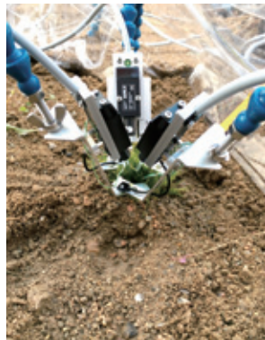
Figure 1. Measurement of photosynthesis of Deschampsia antarctica using the three fluorescence-using instrument
