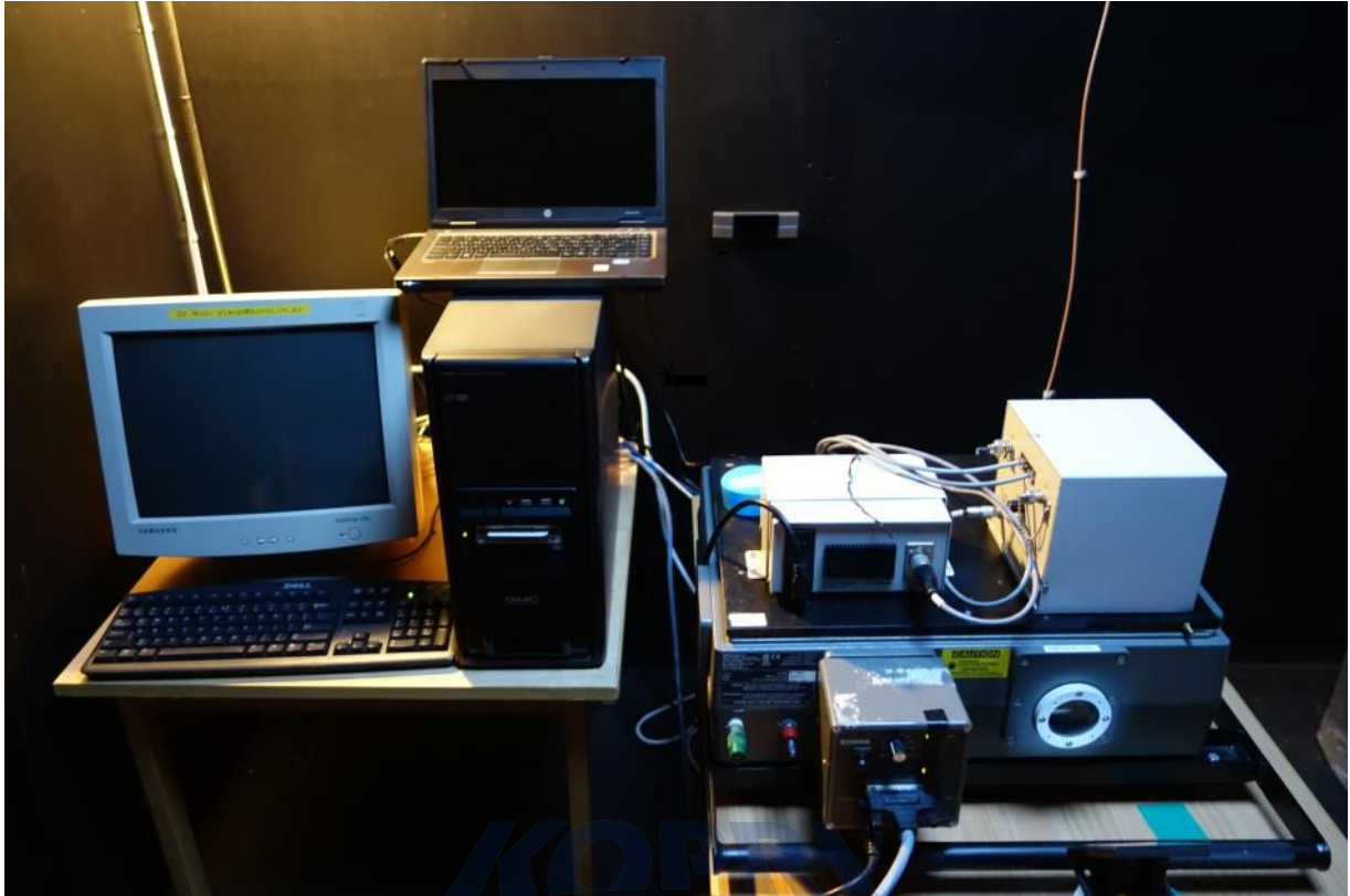
Fig. 53 Fourier-Transform Spectrometer installed at Dasan Station.
