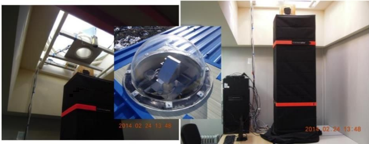
Fig. 50 Fabry-Perot Interferometer (FPI) installed at Jang Bogo Station, Antarctica
