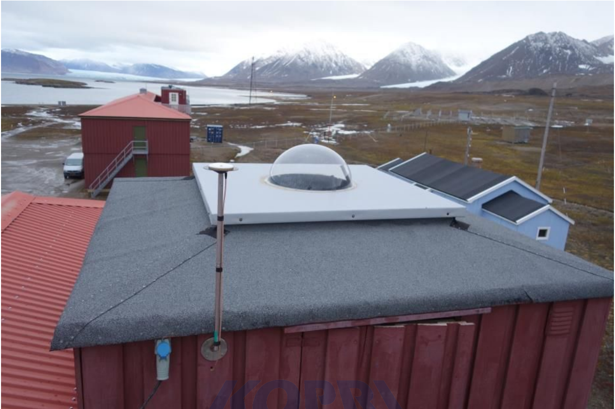
Fig. 54 GPS receiver installed at Dasan Station.
