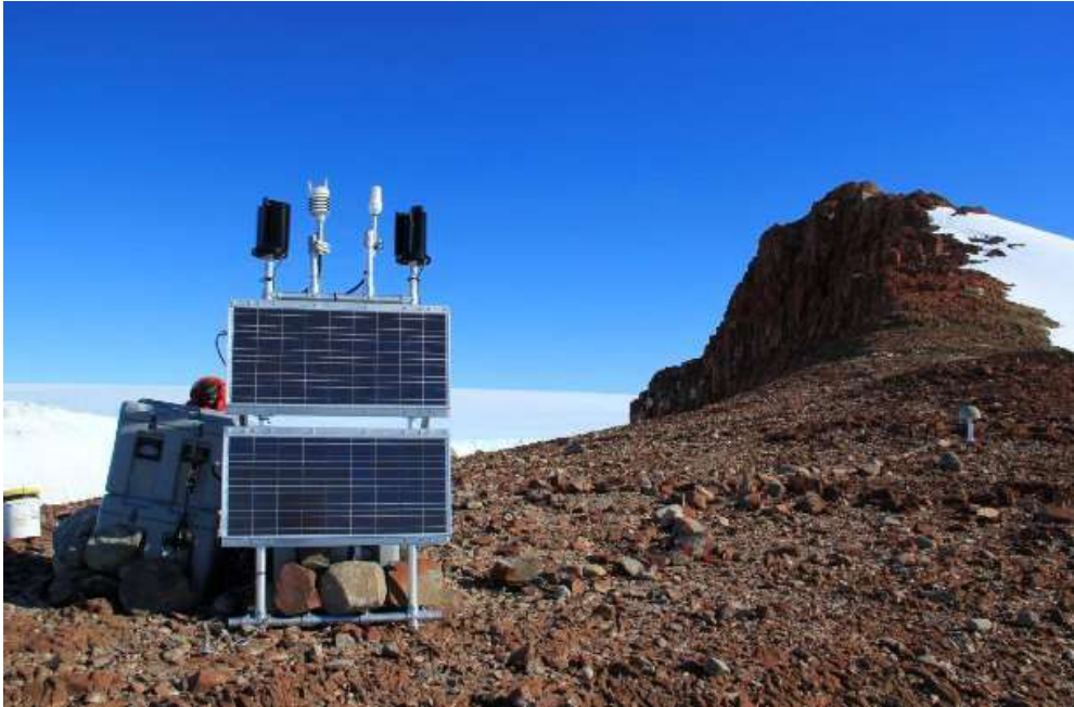
Fig. 37 POLENET GPS station component (1005 kg) (Weather station, Iridium antenna, Battery, Solar panel, High speed wind turbine)
