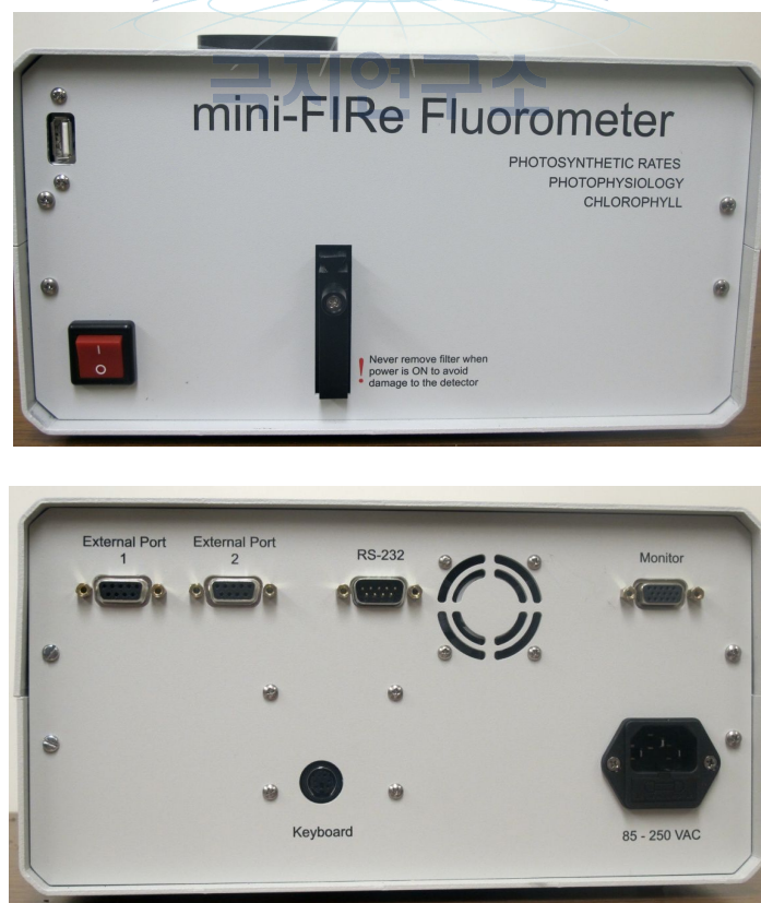
Figure 3. Front and rear panels of the FIRE instrument. (A) The front panel includes the main
