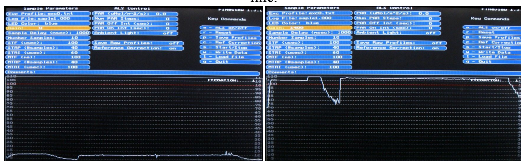
Figure 5. (left) FIRE fluorescence profile with GAIN set too low. (right) FIRE fluorescence profile with GAIN set too high. In the first case the GAIN needs to be increased, in the second – to be decreased.
