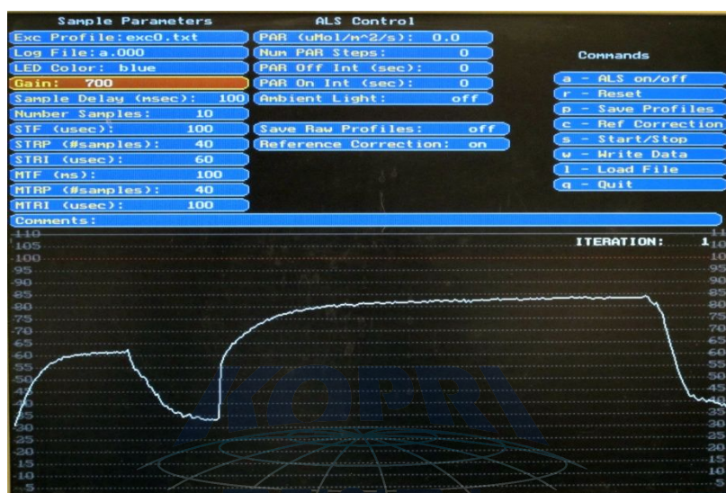
Figure 4. Typical FIRE Fluorescence Profile Acquired with FVIEW Program. Both STF and MTF protocols were used. If MTF is not set (MTF=0 and MTRP=0), only STF Induction and Relaxation will appear in the left part of the screen. GAIN was chosen correctly and the maximum fluorescence level is within the upper 50% or the window and below the red dotted line.
