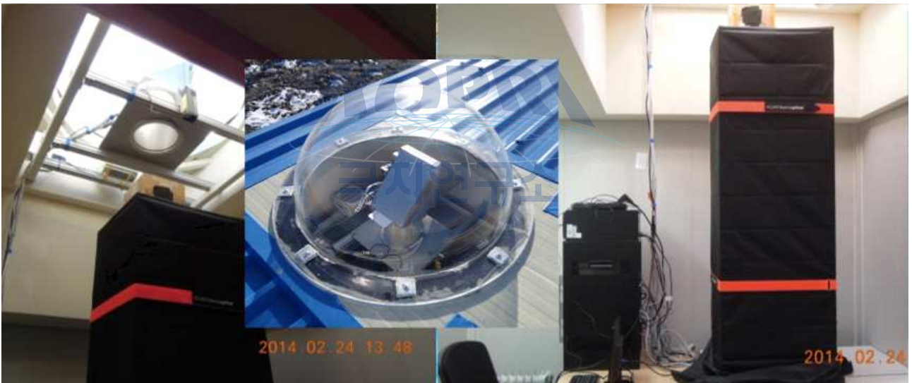
Fig. 15 Fabry-Perot Interferometer installed at Jang Bogo Station, Antarctica in March 2014 to observe the neutral winds and temperature in the polar upper atmosphere.
