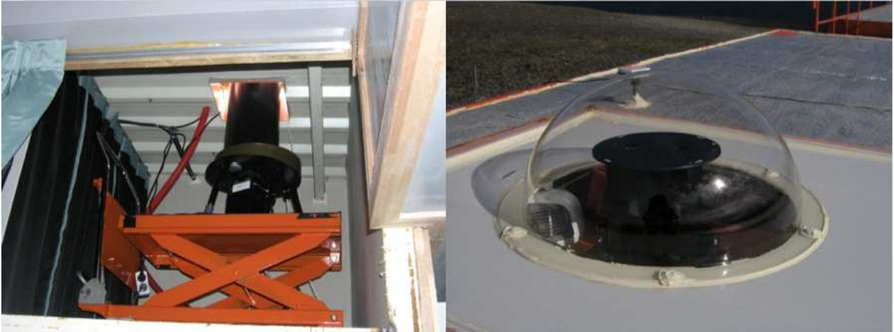
Fig. 11 Spectral Airglow Temperature Imager (SATI) at KSS. It measures airglow emissions occurring at the upper atmosphere to observe the temperature in the region.
