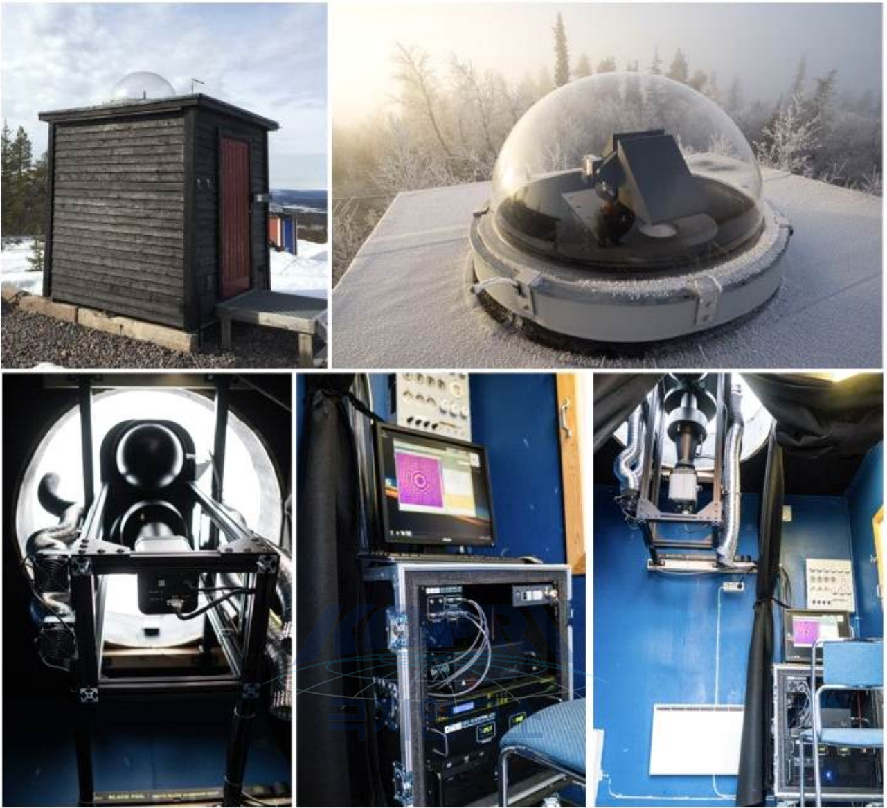
Fig. 22 Fabry-Perot Interferometer (FPI) installed at ESRANGE, Kiruna, Sweden in Oct. 2016 for the simultaneous observations for the neutral winds and ion drift in the auroral region.
