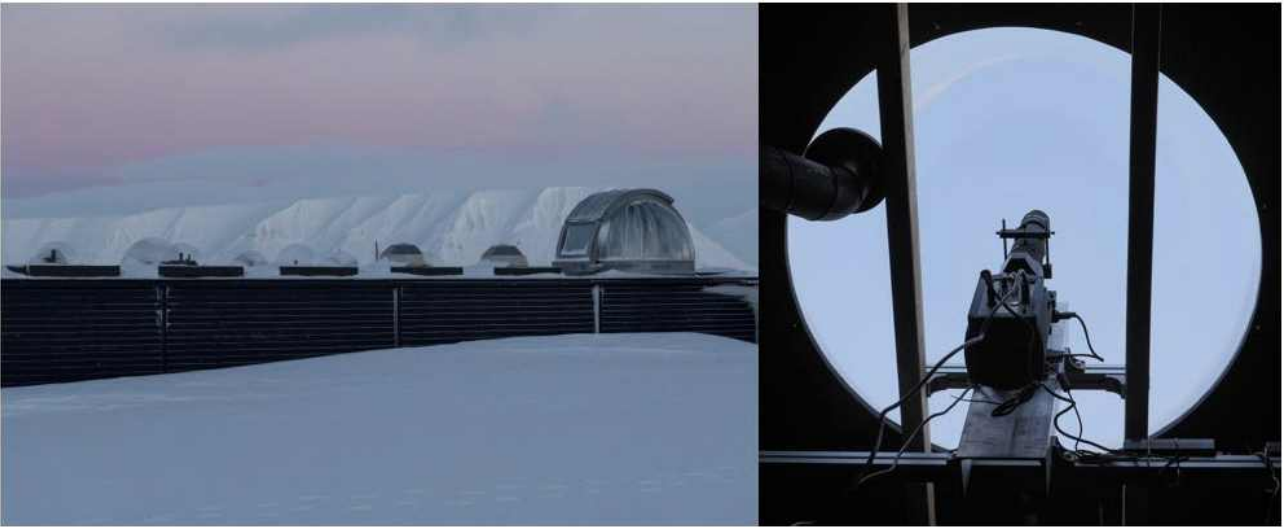
Fig. 23 All Sky Camera installed at KHO, Svalbard, Norway to observe proton aurora near the polar cusp region.
