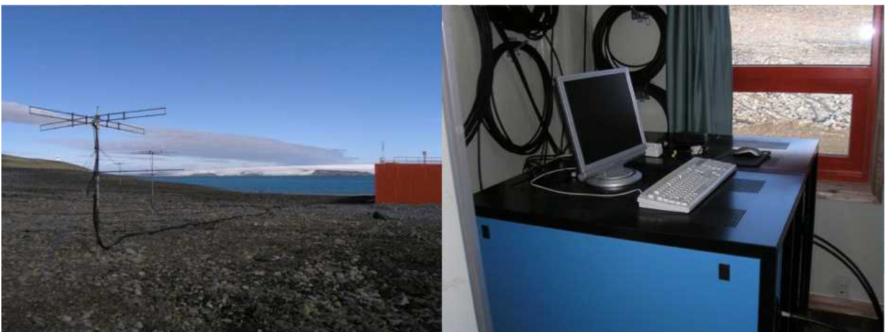
Fig. 12 Meteor Radar at KSS utilizes an electromagnetic wave to observe meteor echoes in order to measure the neutral winds and temperature.
