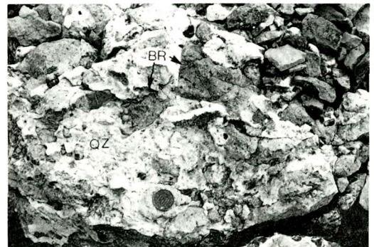
Fig. 7. Hydrothermal vein breccia cemented by silica and pyrite. QZ = quartz, BR = breccia.
