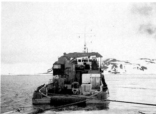
Fig. 3. Pumping up oils from the vessel of EREBUS to tanks installed on land in front of the pier.
