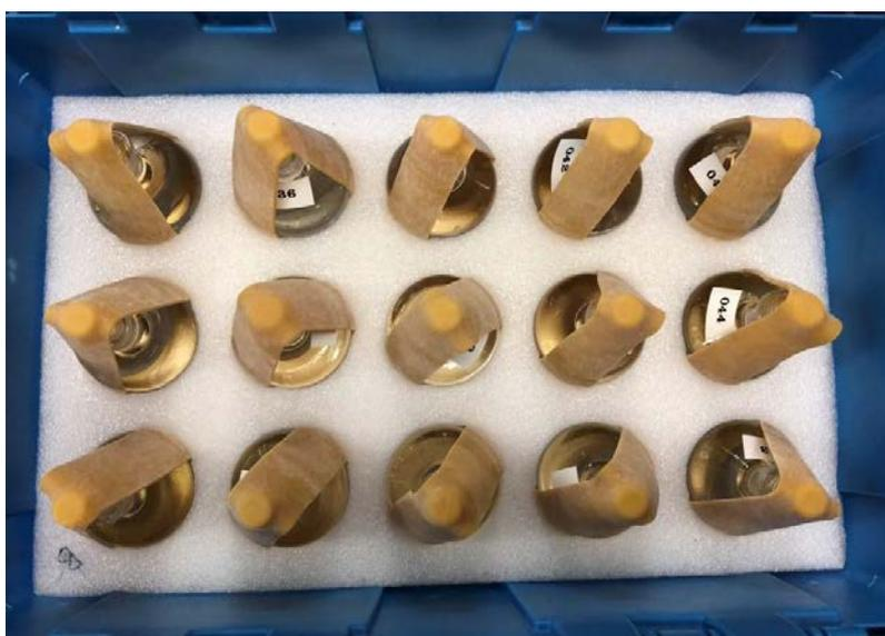
Figure 2.12. Bottled water samples for DIC and TA analysis
