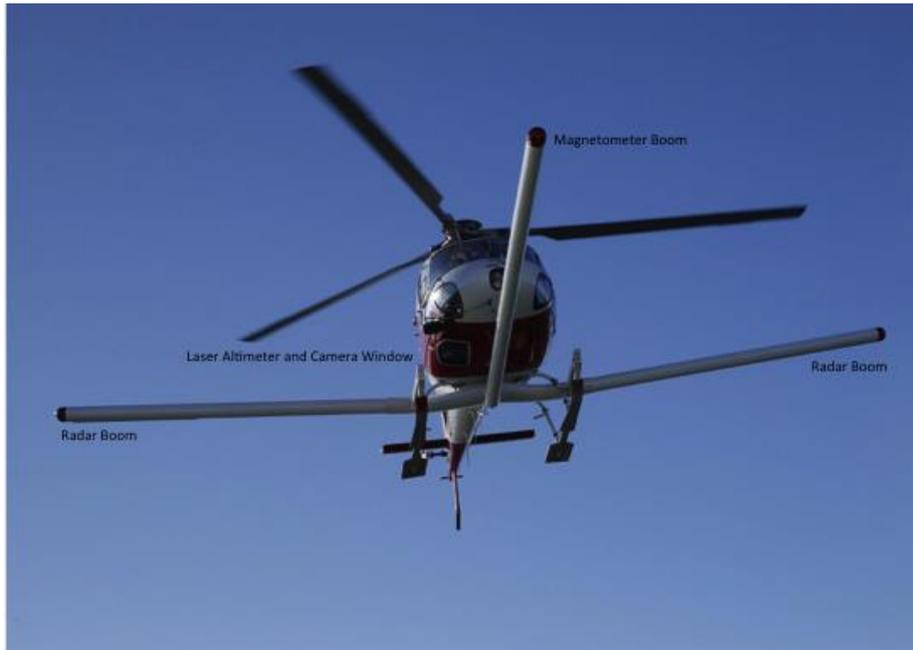
Figure 1.16. Configured survey helicopter with booms.
