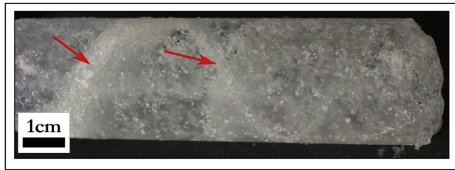
Fig. 2. Photograph of a sub-core as extracted from the main ice core (collected from approximately one metre's depth), showing planes of high porosity (red arrows) emerging on the surface. (For interpretation of the references to colour in this figure legend, the reader is referred to the Web version of this article.)
