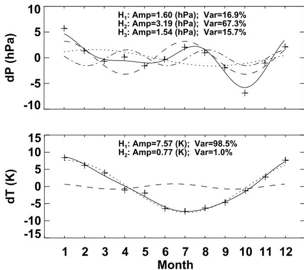
**Figure 12.** Measurements (pluses), the first harmonic  $H_1$  (dotted line), the second harmonic  $H_2$  (dashed line),  $H_3$  (dash-dotted line), and  $H_1 + H_2 (+ H_3)$  (solid line) of mean annual cycles of pressure  $P$  (top) and temperature  $T$  (bottom) for 2008–2014.
