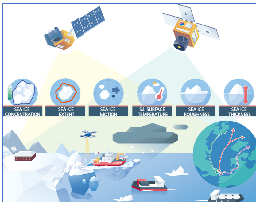
Fig. 2. A schematic illustration on the introduction of scientific research for sea ice at the Arctic Ocean using satellites. Courtesy by Korea polar research institute.
