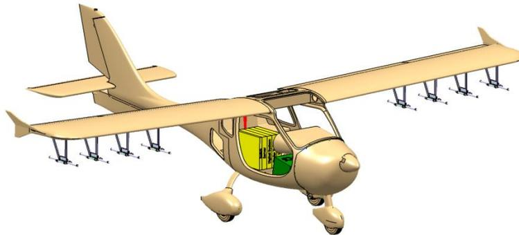
Figure 10. Flight Design CTLS with VHF antennas, pylons, radar systems, and autonomous flight control system
