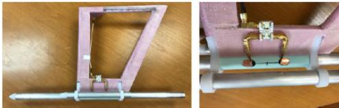
Fig 11. Prototype sleeved dipole antenna
