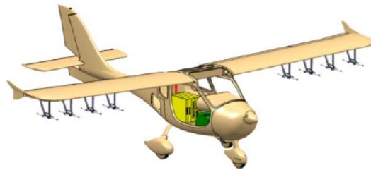
Fig 4. Flight Design CTLS with VHF antennas, pylons, radar systems, and autonomous flight control system
