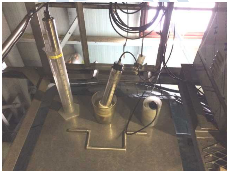
Fig. 6-8. Real time monitoring system(non-reagent) for water quality.
