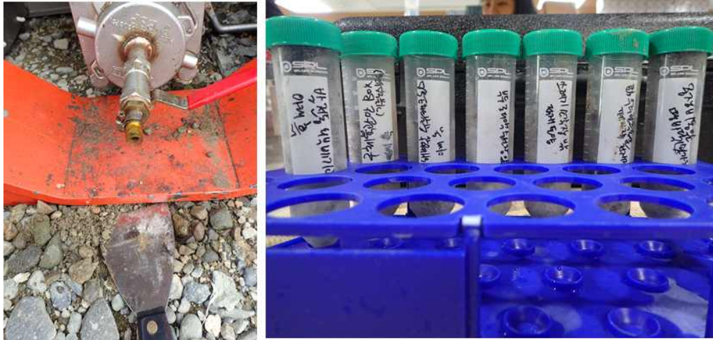
Fig. 9-12. Fuel spill from ISO tank valve (left) and collected soil samples.
