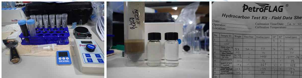
Fig. 9-13. TPH test results of oil contaminated soil at the laboratory in King Sejong Station.
