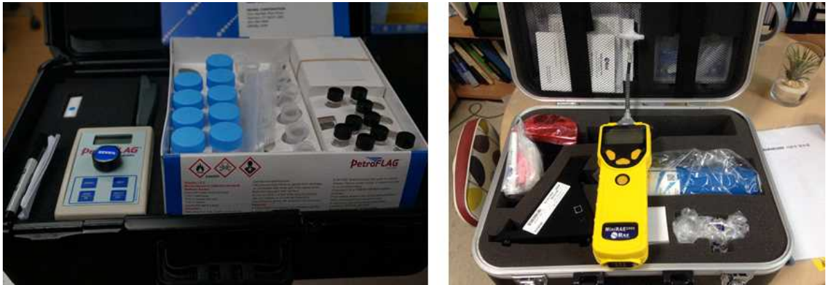
Fig. 9-2. Portable oil spill detecting equipment. PetroFLAG Kit (left) to detect TPH and minRAE 3000 (right) to detect VOCs.
