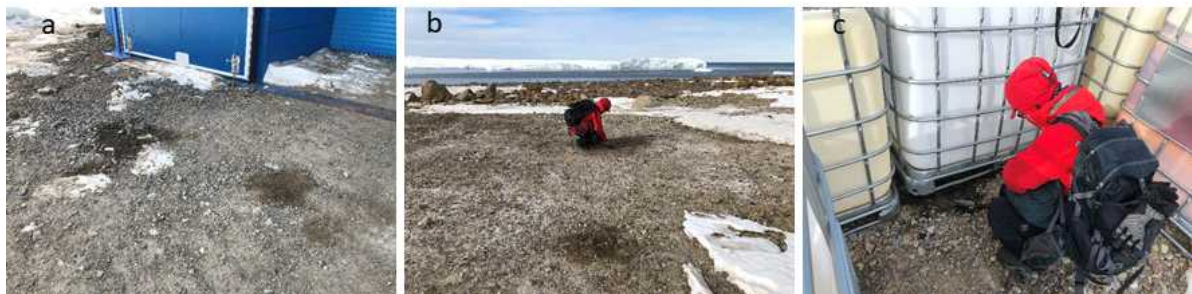
Fig. 9-5. Fuel spill spot near maintenance building and helipad. a. spots in the front of maintenance building, b. spots on helipad, c. waste aviation fuel spill.
