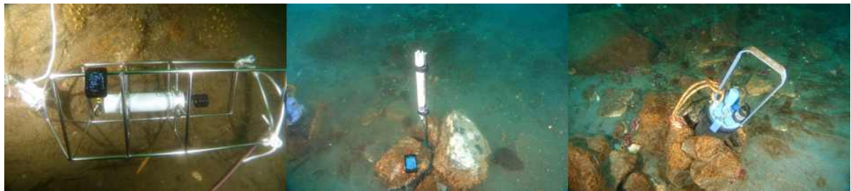
Fig. 3-17. CTD and water temperature sensor installed in water.
