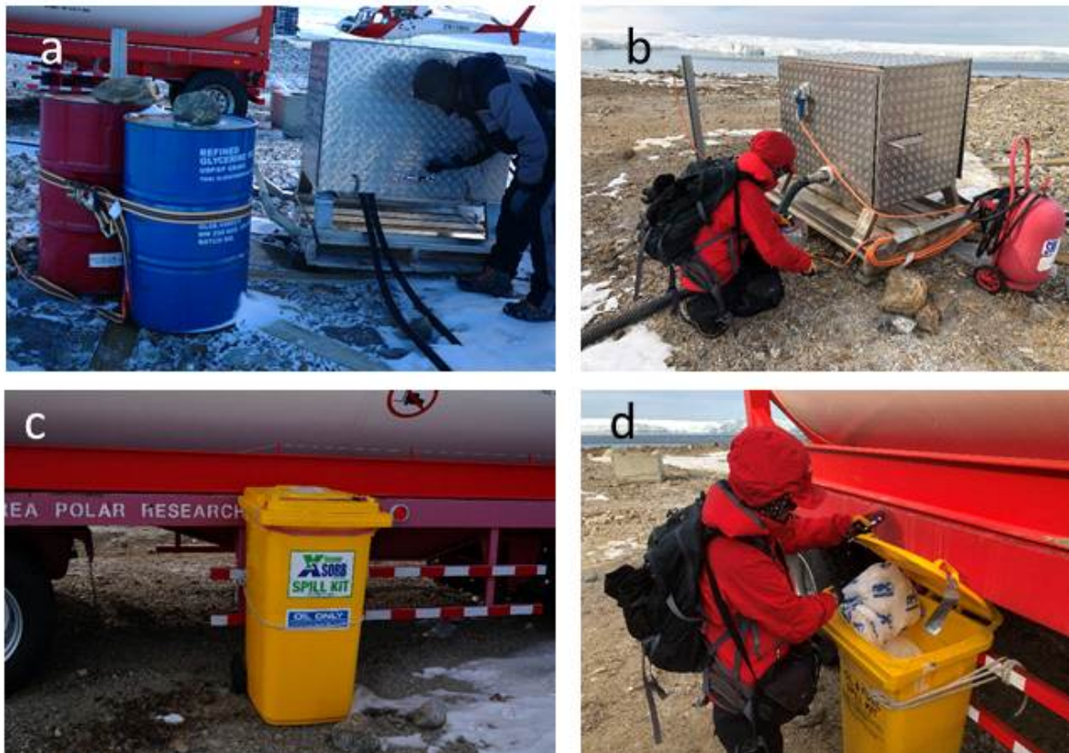
Fig. 9-3. Fuel handling at helicopter landing pad. a. service tank near by empty fuel drum to recover remaining fuel in the hose, b. inspection of fuel spill, c, d. container for fuel spill adsorbent
