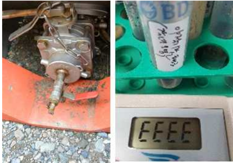
Fig. 9-10. Fuel spill from ISO tank valve (left) and collected soil samples with error message of photometer showing error message due to beyond resolution of the photometer.
