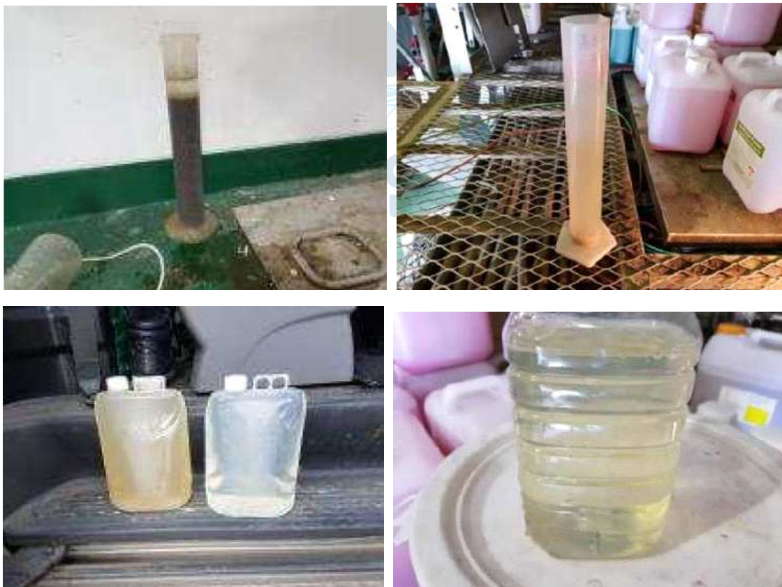
Fig. 5-4. Colour comparison of general domestic sewage (left) and King Sejong Station sewage (upper right: SV30, bottom: discharged water)
