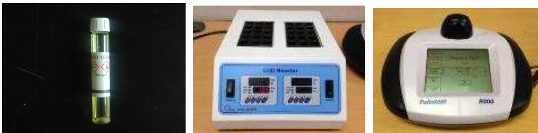
Fig. 2-14. Palintest COD detection kit. Tubetests COD tube(left), heater(center), wavelength selection photometer(right).
