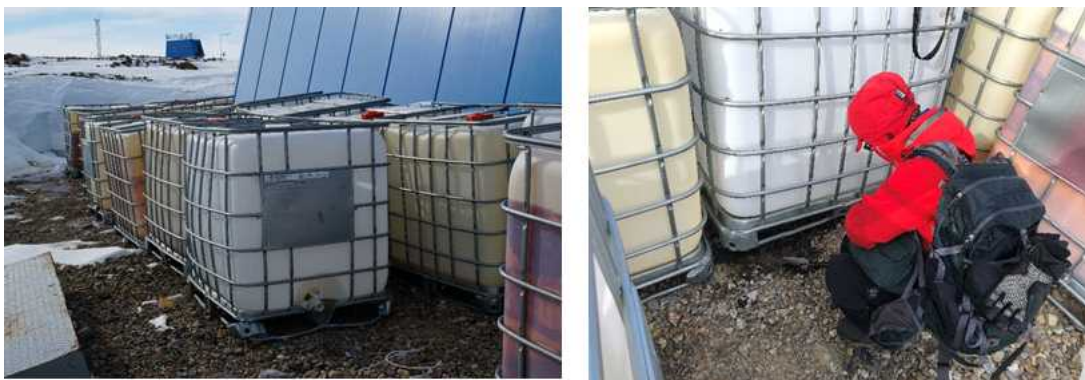
Fig. 1-7. Waste aviation fuel storing tanks (left) and collecting contaminated soil beneath the tanks (right) in March 2019.
