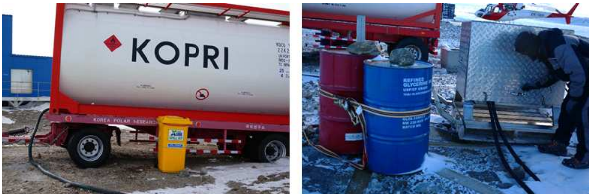
Fig. 2-13. ISO fuel tanks for aviation fuel next by spill kit (left) near helipad and waste fuel drum next by fuel service equipment(right).
