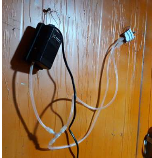
Fig. 8-6. Collecting the olfactory-active compounds for WCF using dynamic headspace collection system installed in sewage inlet building near accommodation building.
