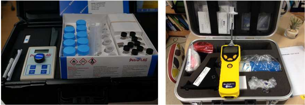
Fig. 1-2. Portable oil spill detecting equipment. PetroFLAG Kit (left) to detect TPH and minRAE 3000 (right) to detect VOCs.
