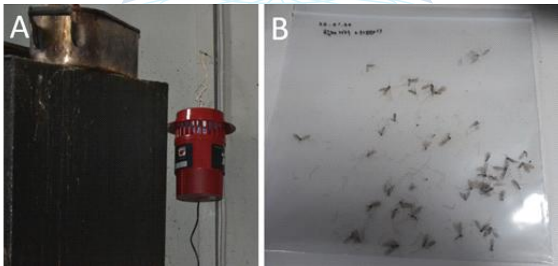
Fig. 8-24. UV trap (A) installed in sewage collecting site and captured WCF adults by the trap (B).
