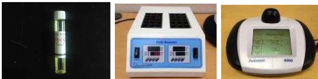
Fig. 3-12. Palintest COD detection kit. Tubetests COD tube(left), heater(center), wavelength selection photometer(right).
