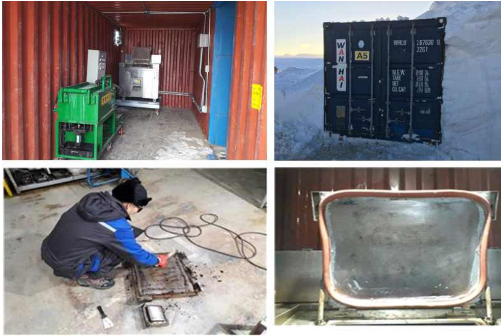
Fig. 2-3. Waste treatment facility using 20ft container (upper) and maintenance of food waste processor (below).
