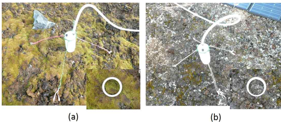
Figure 5. Two FD chambers for soil CO 2 efflux in KGL01 site. (a) moss, (b) lichen.
