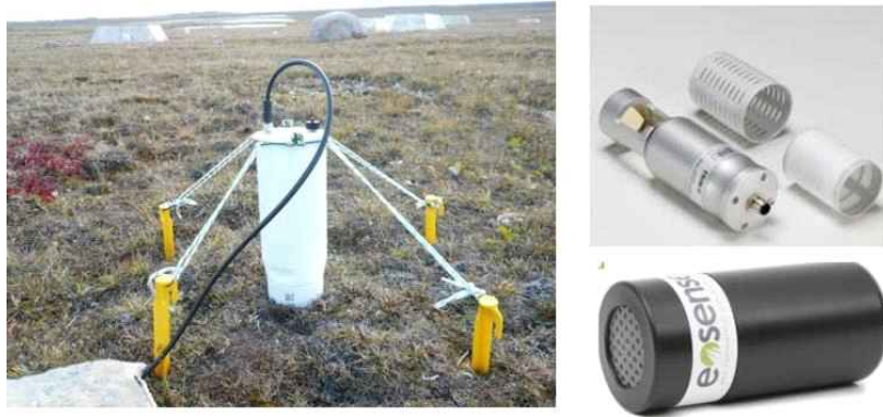
Figure 1. Chamber and sensors for CO 2 monitoring [Left, FD chamber; Right up, CO 2 concentration probe(GMP 343); Right down, CO 2 concentration probe(GP sensor)]
