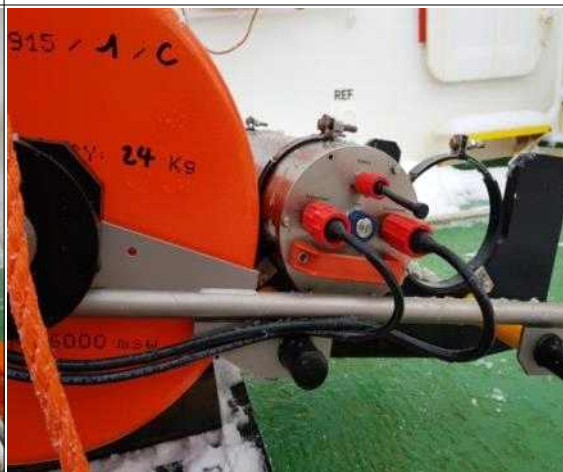
OBS ON THE DECK
