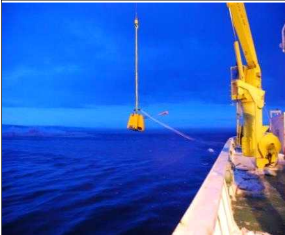
OBS DEPLOYMENT BY 3TON CRANE
