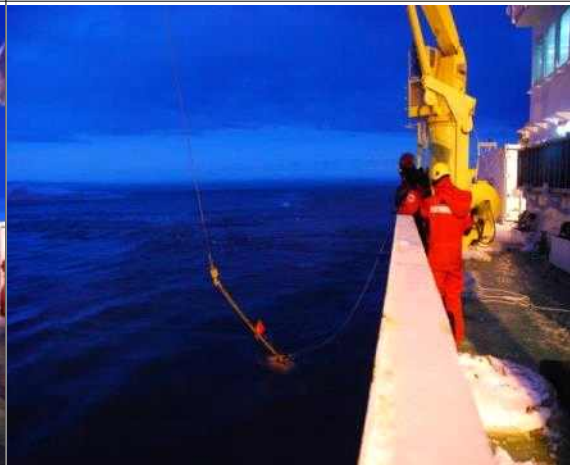
OBS DEPLOYMENT BY 3TON CRANE
