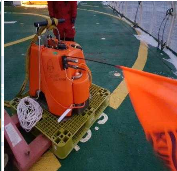
OBS SETTING ON THE POOP DECK
