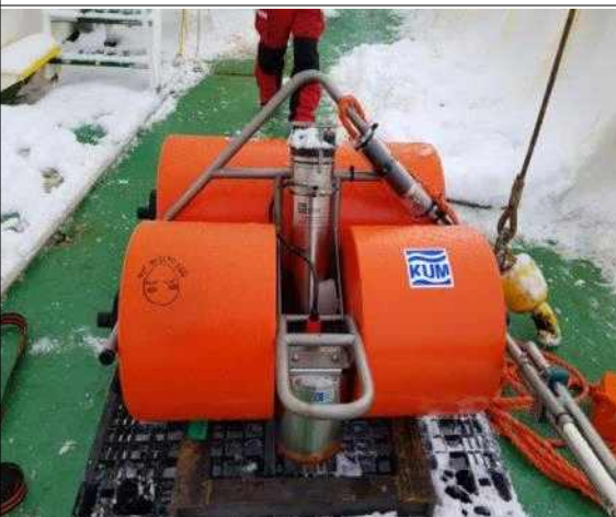
OBS ON THE DECK
