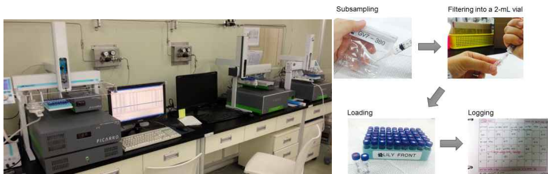
그림 3.1.2 Cavity RingDown Spectrometers, L1102-i, L2140-i and L2130-i, Picarro; Right: Sample preparation for the autosampler vials
