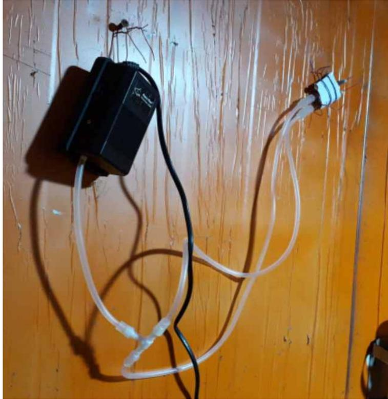
Figure 3-14. A dynamic headspace volatile collection system to collect volatile organic compounds (VOCs) produced in the sewage collection facility receiving sewage water from the main building at King Sejong Station. This area is a main breeding site of winter crane flies in the station.
