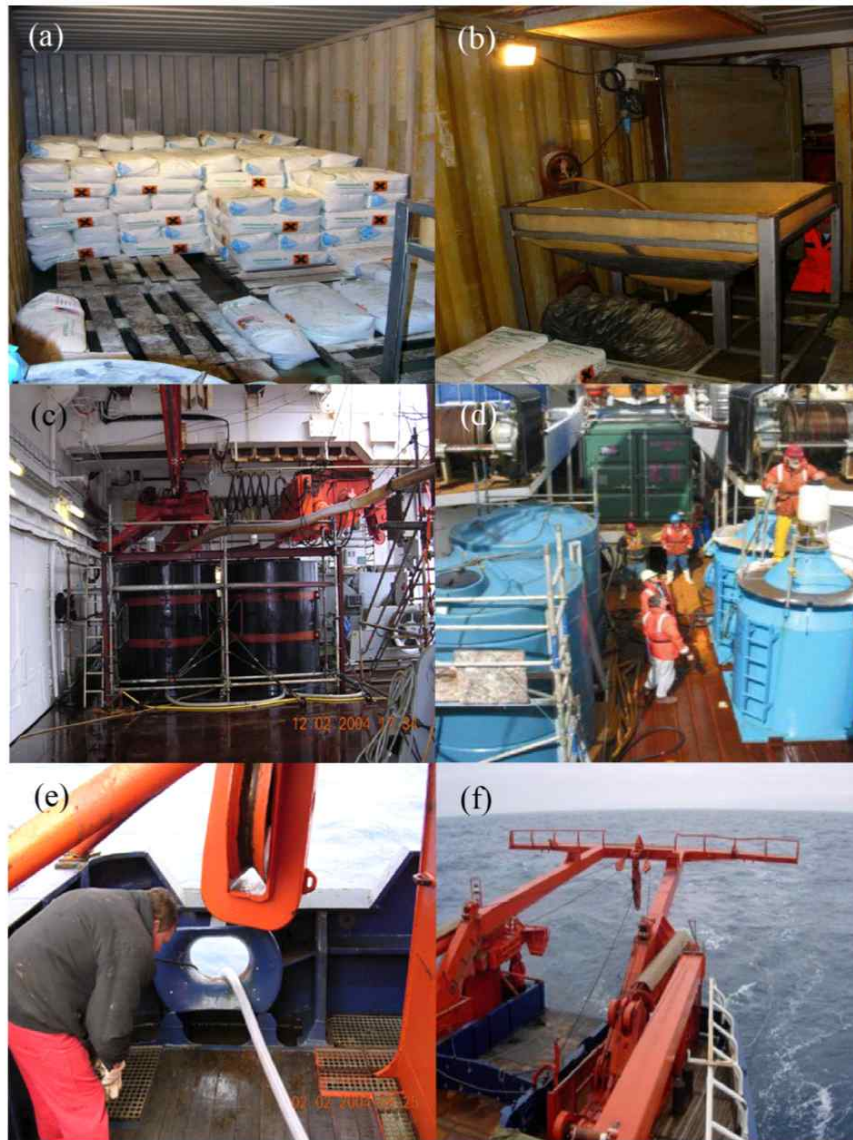
Figure 5. Photographs of the iron addition procedure. Panels a–f taken during the European Iron Fertilization Experiment (EIFEX), Surface Ocean Lower Atmosphere Study (SOLAS) Air - Sea Gas Exchange (SAGE), and Indo-German iron fertilization experiment (LOHAFEX): (a) Iron (II) sulfate bags. (b) The funnel used to pour iron and hydrochloric acid. (c) Tank system used for mixing Iron(II) sulfate, hydrochloric acid, and seawater (Smetacek, 2015). (d) Preparation for release: the deck of RV Tangaroa with the iron tanks on the left and the SF 6 tracer tanks on the right (Photo: Matt Walkington). (e) Outlet pipe connected to the tank system. (f) Pumping iron into the prop wash during EIFEX (Smetacek, 2015).
