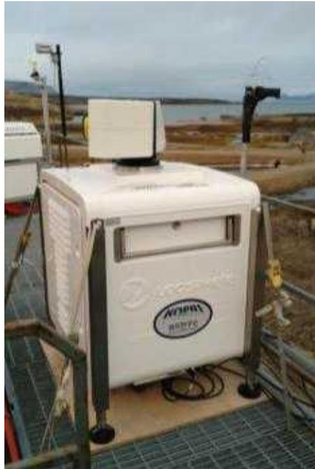
Figure 3.1.9 Doppler Wind Lidar installed on the roof of German station at Ny-Alesund, Svalbard.
