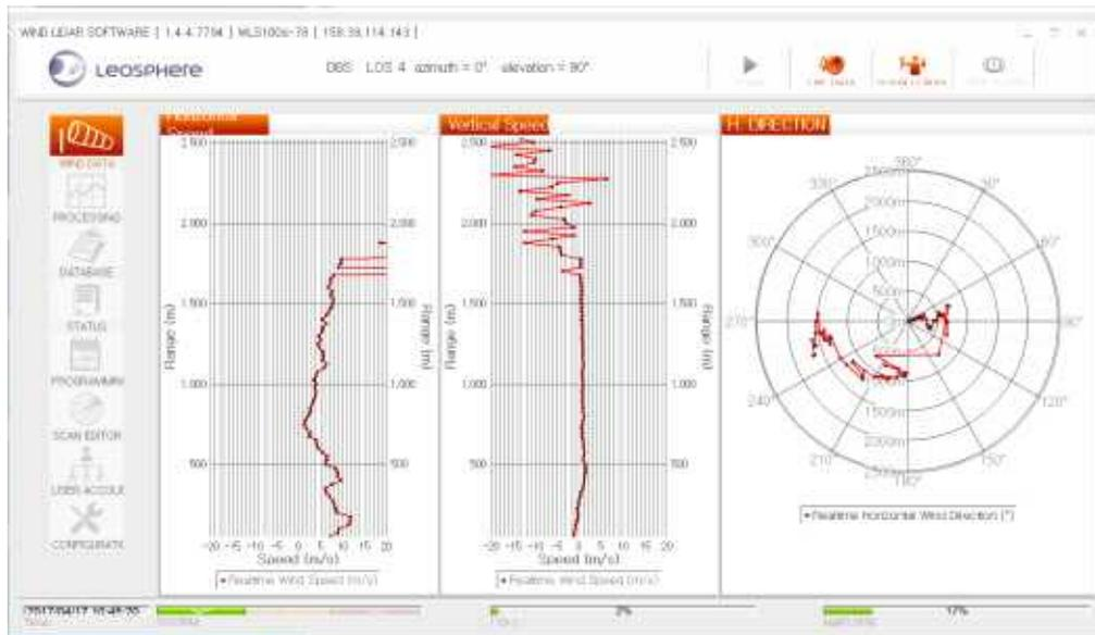
Figure 3.1.14 Screenshot of DBS-mode of the wind lidar.
