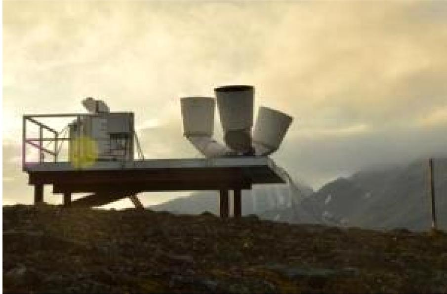
Figure 3.1.22 Wind lidar(left) and SODAR(right) at Ny-Alesund, Svalbard (September 2018).
