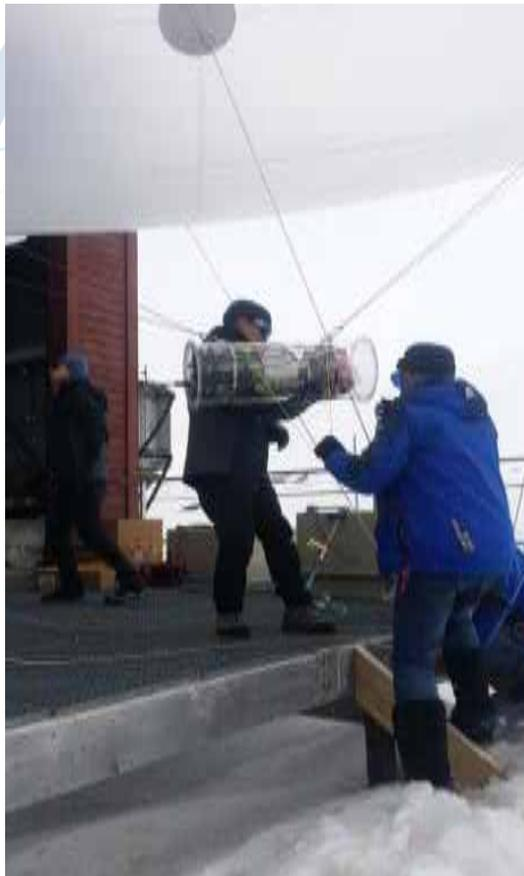
Figure 3.1.29 Attachment of the cloud probe under the tether-balloon.
