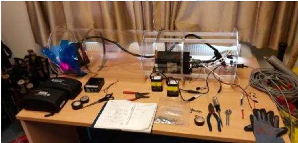
Figure 3.1.27 Backscatter cloud probe (BCPD) under assembly for tether-balloon operation at the Ny-Alesund, Svalbard.
