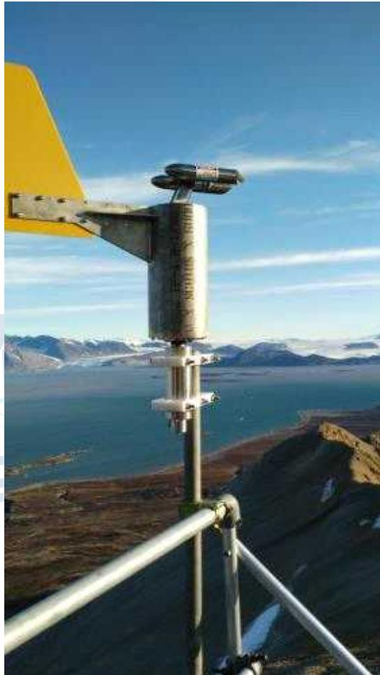
Figure 3.1.19 A cloud droplet probe (CDP-2) on the roof of the Zeppelin observatory (September 2017).
