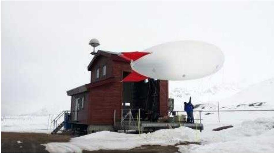
Figure 3.1.28 Italian tether-balloon on the ground before in-cloud measurement.
