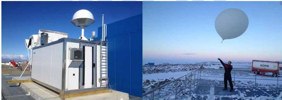
Fig. 3.2.10. Automatic (left) with Autosonde (AS15) and manual radiosonde launch
