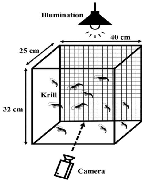
**Fig. 2.** Experimental water tank used for the photographing method for the swimming orientation measurement and image system
