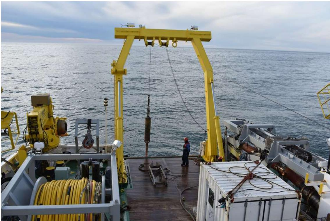
Fig. 19. Sediment coring by a gravity corer (GC) during ARA09C Expedition
