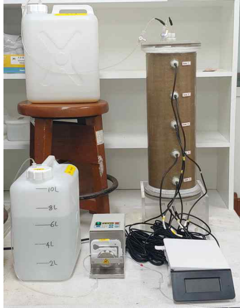
Figure 2.1.1. Photograph of the laboratory experimental setup for the soil column saturation test.
