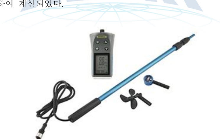
Figure 1.1.10. A flow meter used to measure surface water flow rate.
