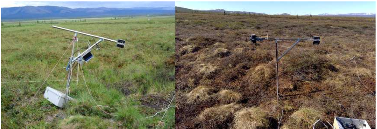
Fig. 4. (Left) Previous version LED sensor in spring season. (Right) Newly installed LED sensor on 2019
