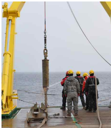
Figure 8. Sediment coring by A) a multicorer (MC) and B) a gravity corer (GC) during the ARA09C Expedition in 2018.
