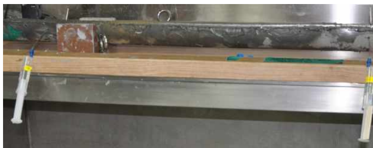
Figure 9. Pore fluid extraction by Rhizon during the ARA08C Expedition.
