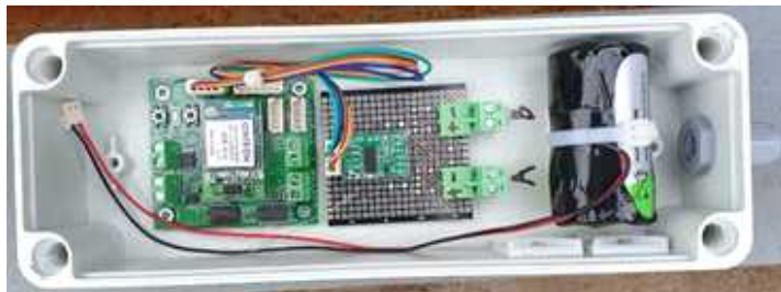
Fig. 6. Electrical resistance strain gauge interface board.
