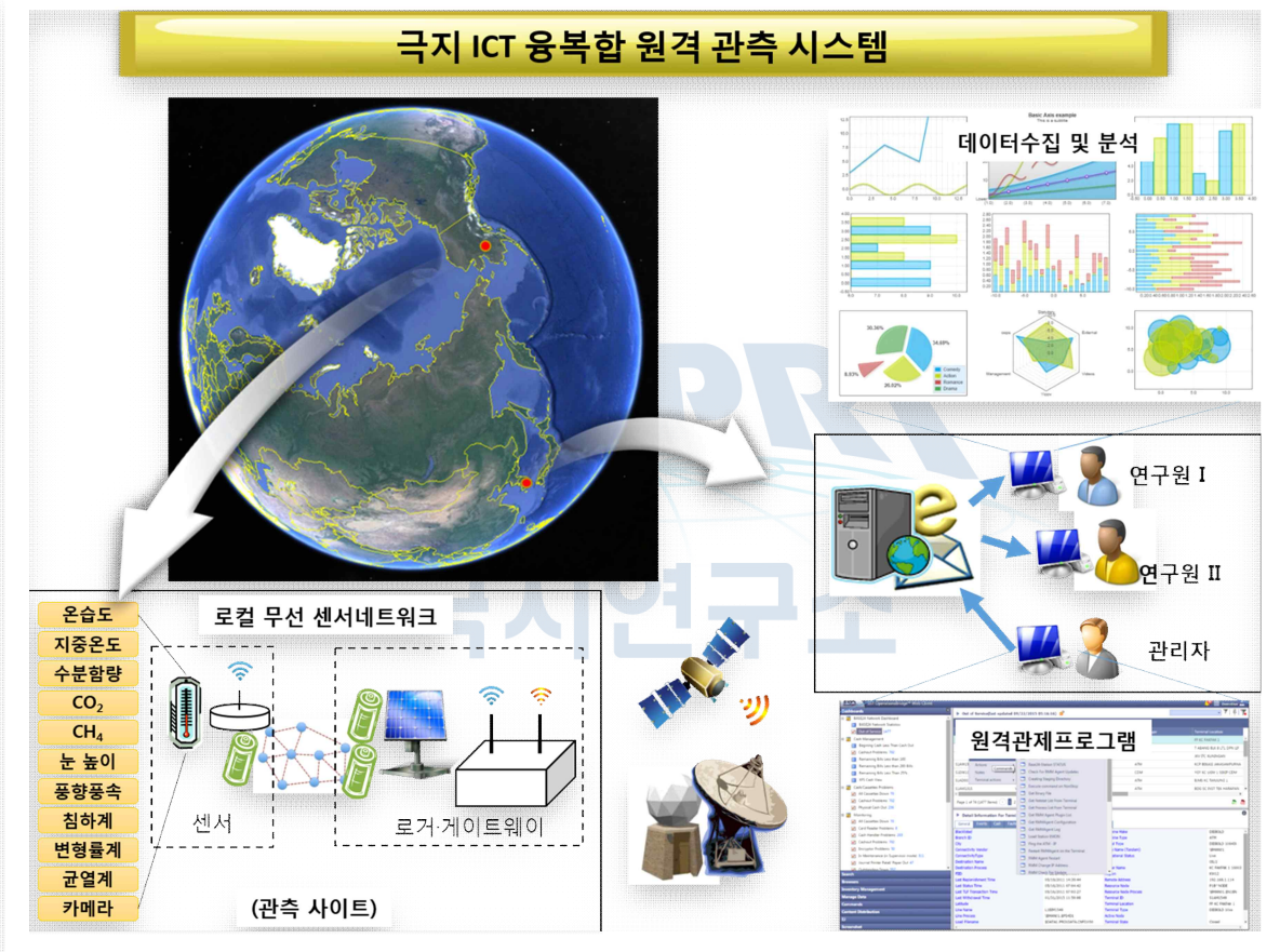
Fig. 1. ICT Based Polar Environment Monitoring System.
