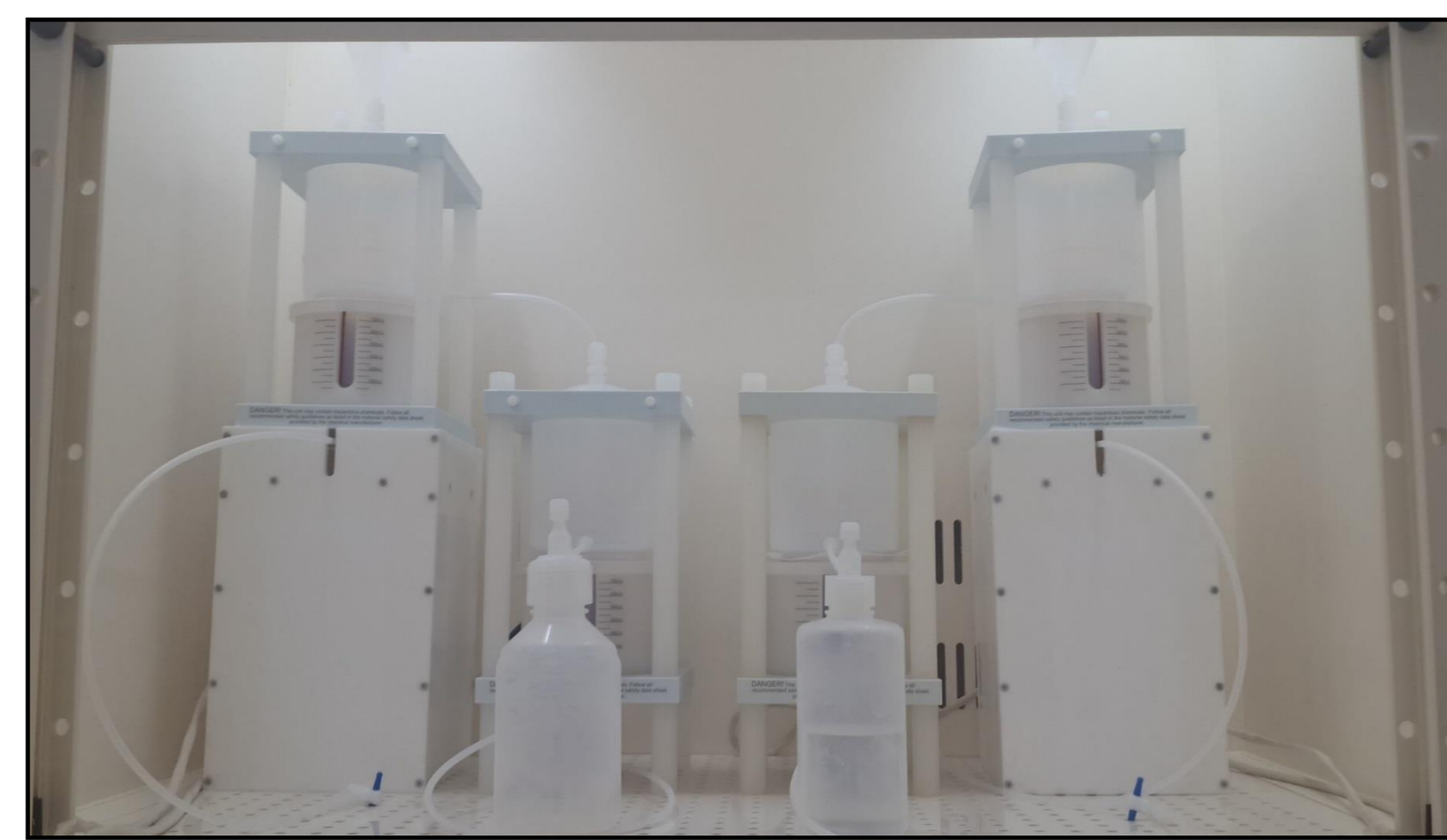
Figure 7. Double distillation Sub-boiled System (DTS-1000 Sub-boiling distillation system, Savillex)
