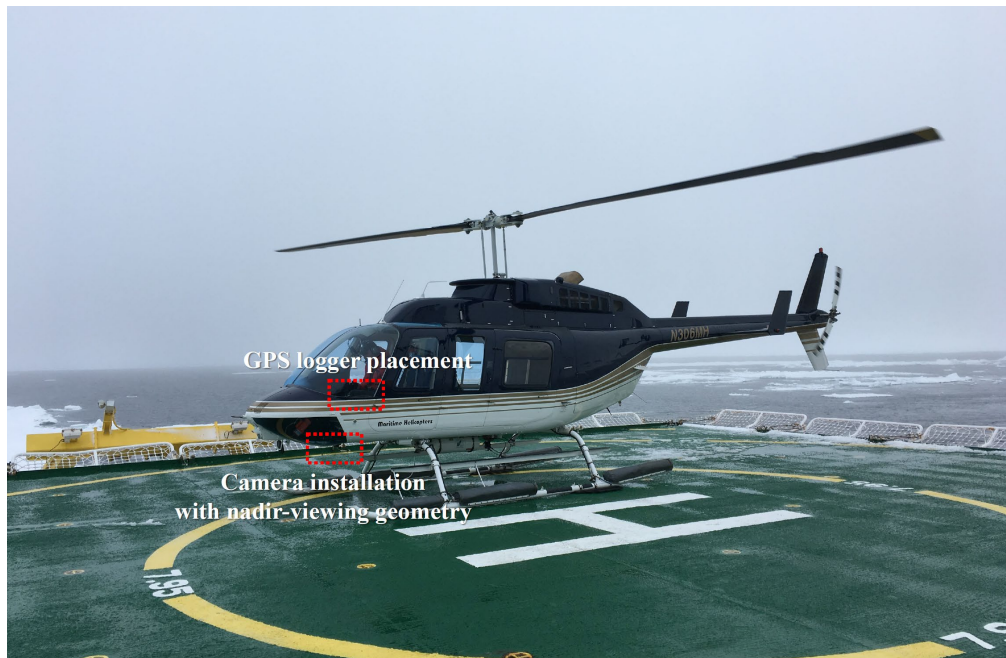
Figure 2. Details of the installation of the imaging equipment and GPS logger on the helicopter carried on board the IBRV Araon.
