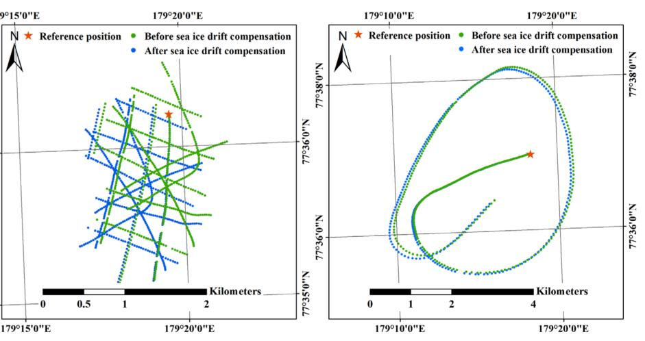
Errors were estimated from camera location of the subsets before and after sea ice drift compensation during image mosaicking processes.
