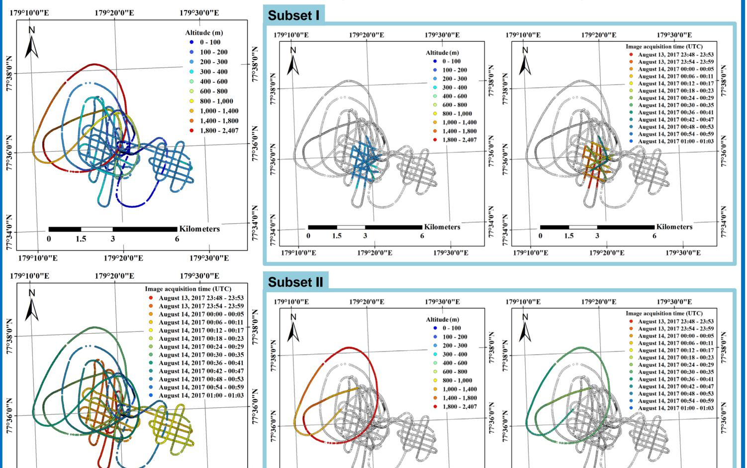
In a post-processing procedure, the GPS logs of the time difference less than 0.02 second between GPS log and timing of image acquisition were selected and designated as the image acquisition positions of corresponding images.
