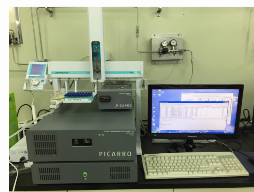
Fig 3. The water isotope analyzer, CRDS(Picarro-L2130) in KOPRI
